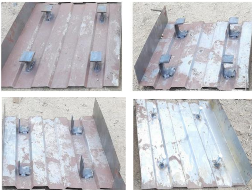
Figure 3 Steel decking sheet with welded shear connectors
