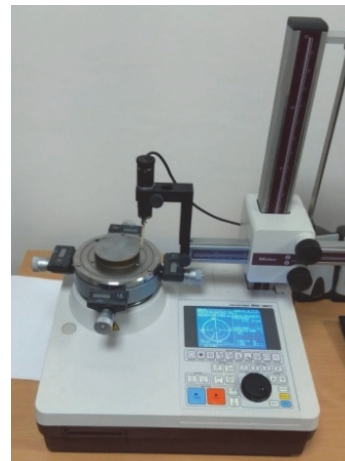
Figure 4 Measurement of circularity deviations y_{Cmax} of experimentally prepared samples using compact MittestoyRoundtest RA-120 measuring instrument
