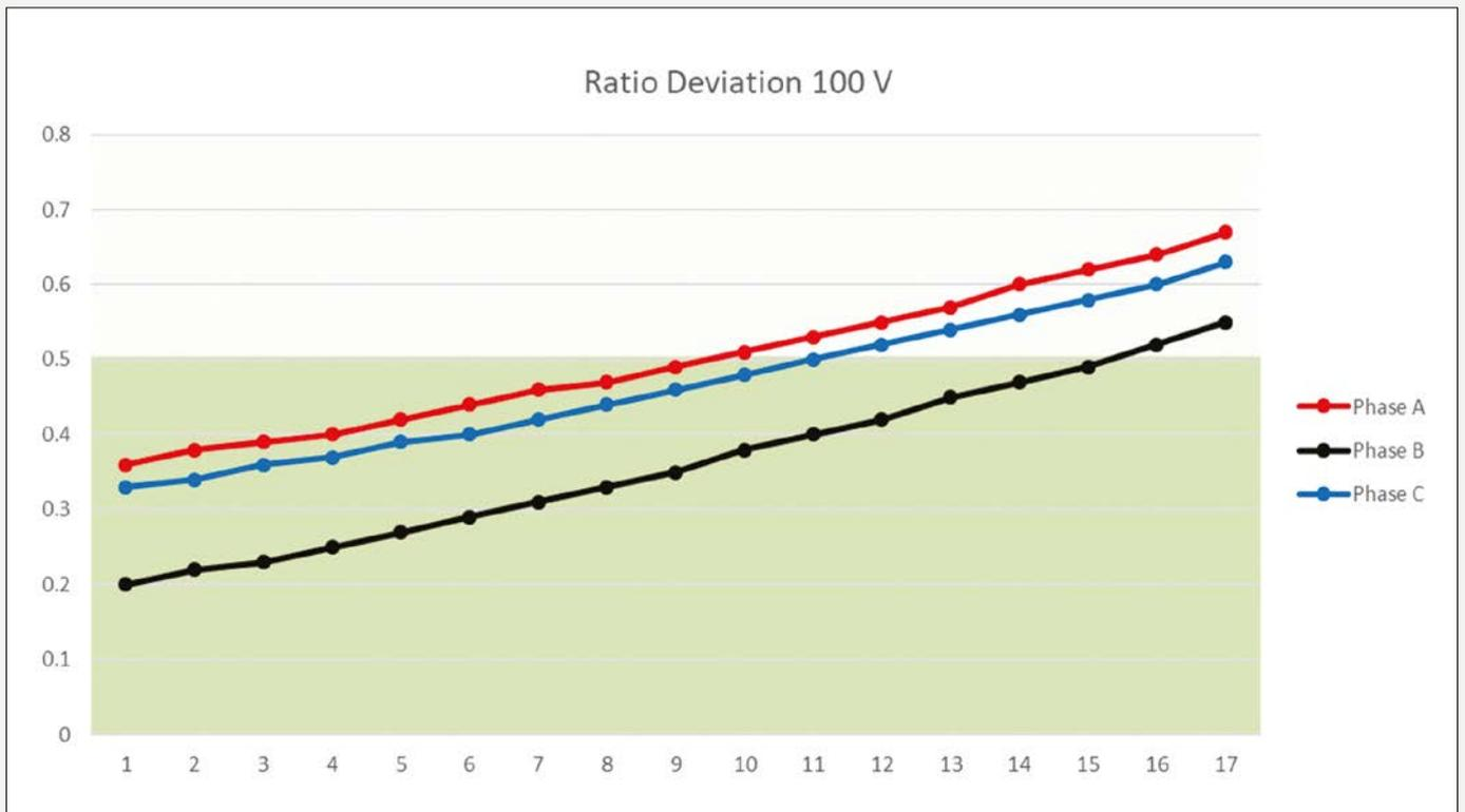
Figure 5. Turns ratio deviation vs. tap positions graph. The green area is a "pass zone" within  $\pm 0.5\%$
