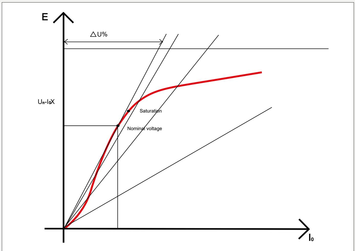
Figure 3. Transformer saturation curve dependent on the no-load current is not linearly decreasing with the voltage decreasing
