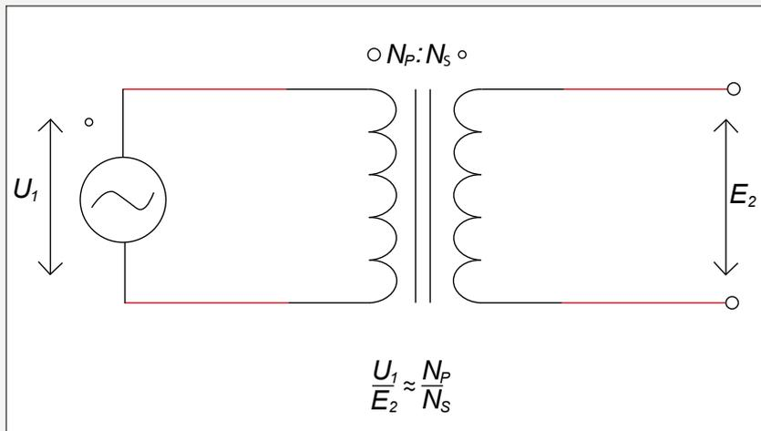
Figure 1. Transformer turns ratio measurement
