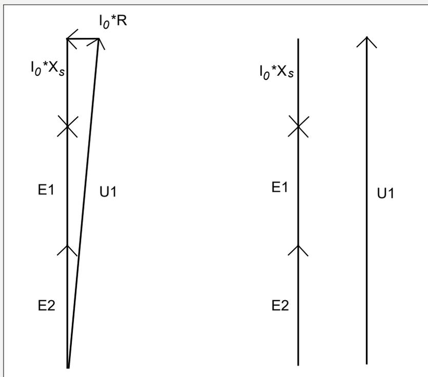
Figure 2. Voltage drop crated by inductive no-load current involves the turns ratio measurement error
