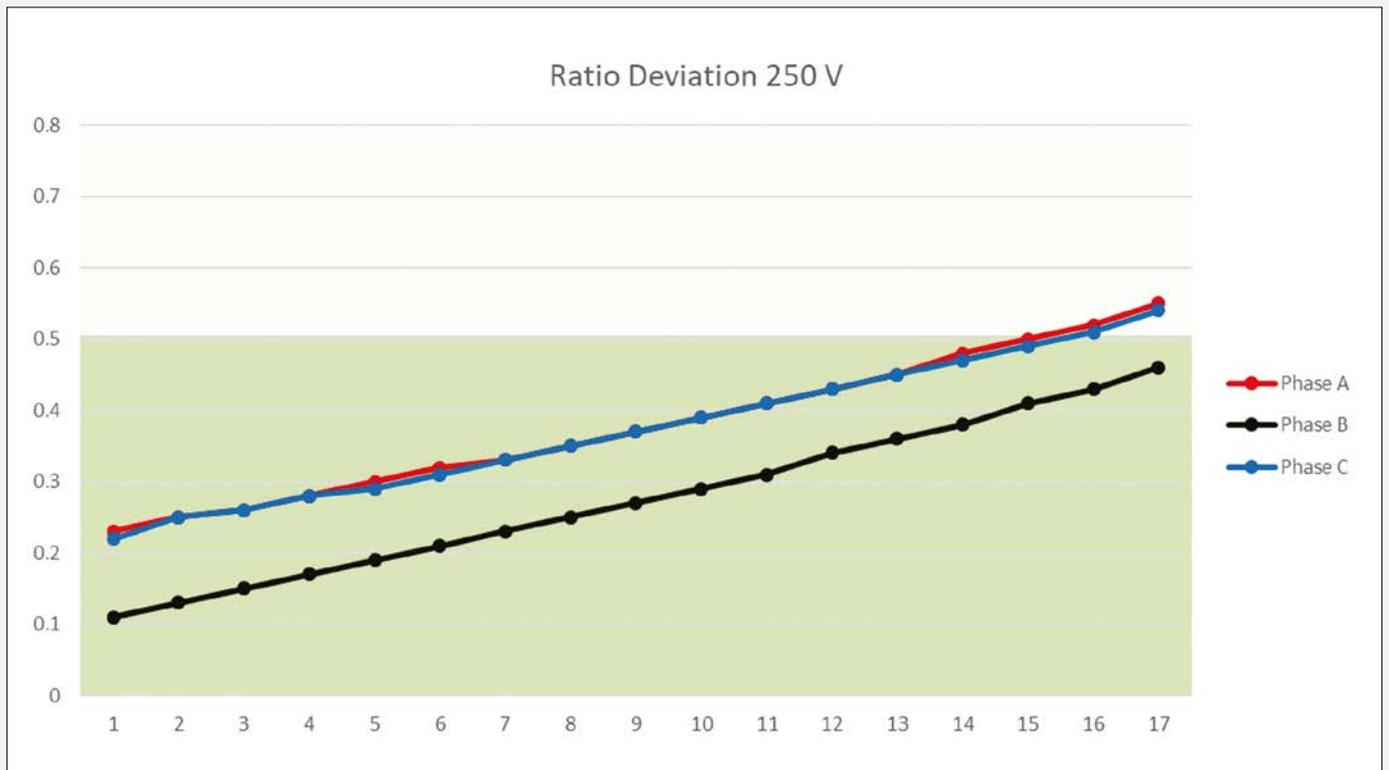
Figure 6. Turns ratio deviation vs. tap positions graph. The green area is a "pass zone" within  $\pm 0.5\%$
