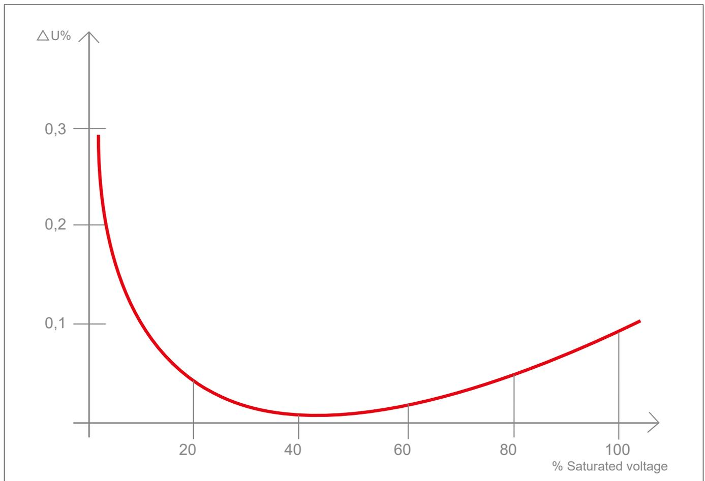
Figure 4. The measurement error vs test voltage curve
