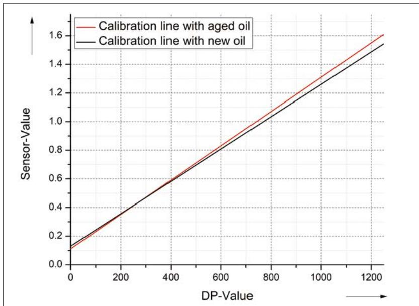
Figure 8. Calibration lines recorded under aged and new oil.
