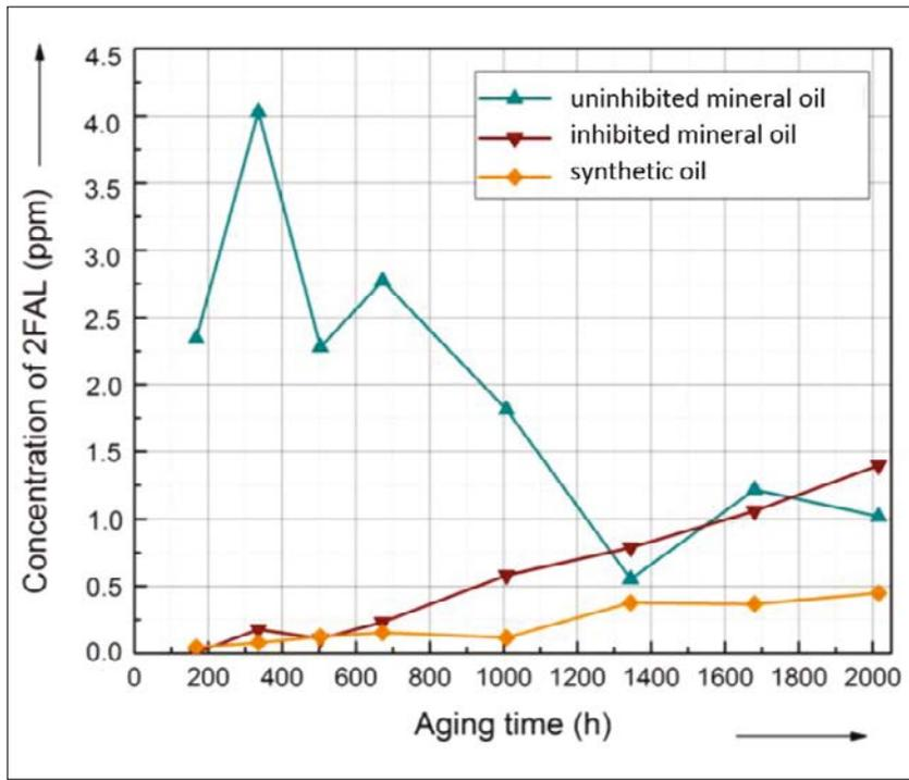
Figure 2. The concentration of furanic compound 2-FAL vs. aging time for different oils in the aging process of oil-paper insulation [11]
