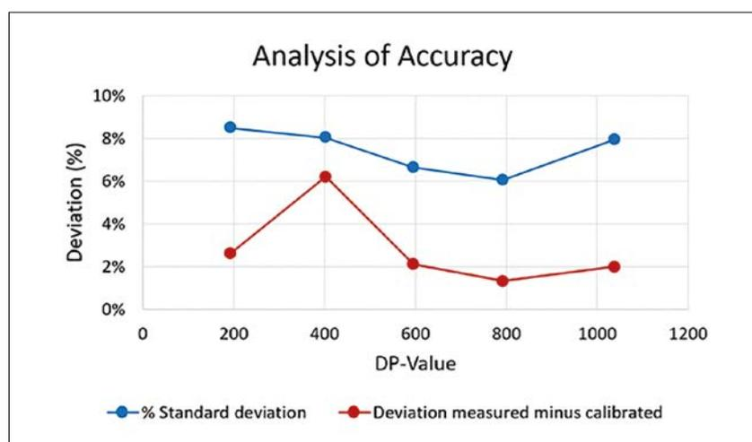
Figure 13. Deviation analysis of DP-value measurement: percentage of the standard deviation of 50 test points and deviation between measured and calibrated value
