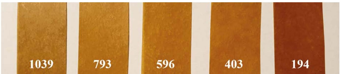
Figure 11. Aged insulation papers calibrated for DP between 1039 and 194 by viscometric analysis according to IEC 60540 (calibrated DP-values shown in the figure)
