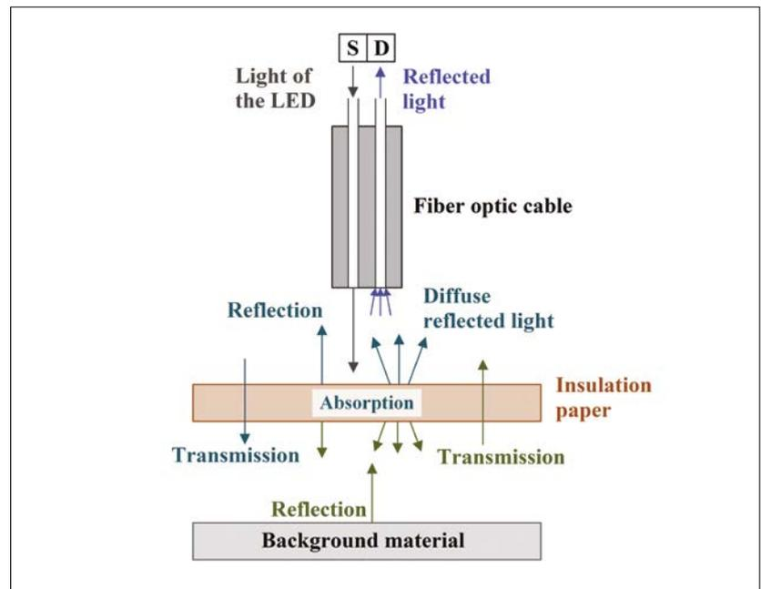
Figure 4. Schematic setup of the sensor head and path of light during the measurement
