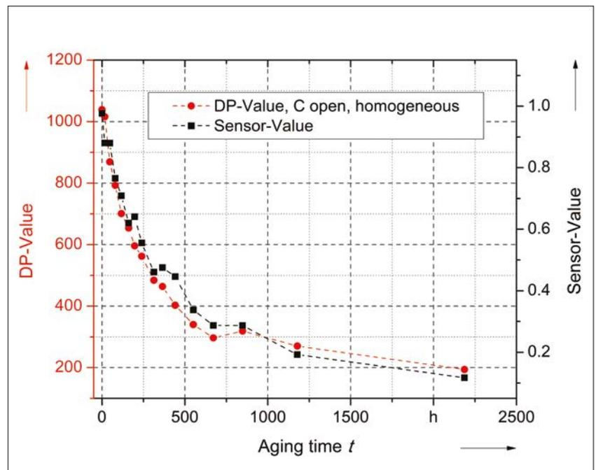
Figure 6. Measured DP-value (red) via viscometry and measured sensor value (black) over aging time for Oil C in an open system with a homogeneous arrangement
