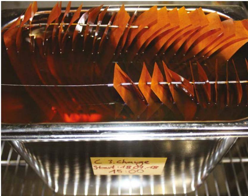
Figure 5. Arrangement of oil-paper samples during thermally accelerated ageing in the oven
