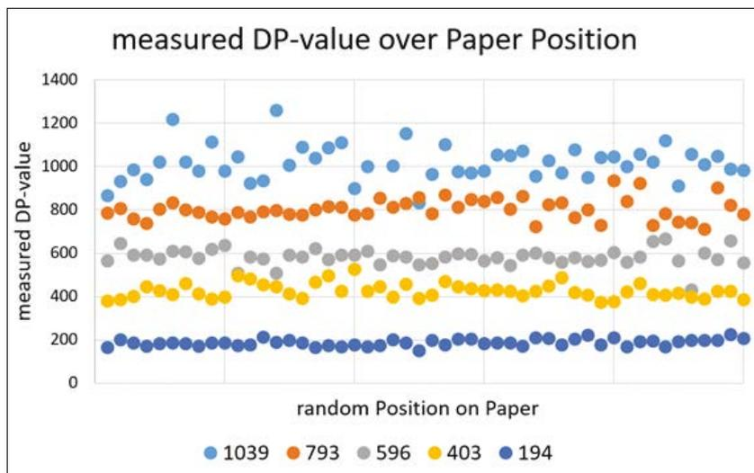
Figure 12. Test results on 50 randomized positions on different aged and calibrated insulation papers.
