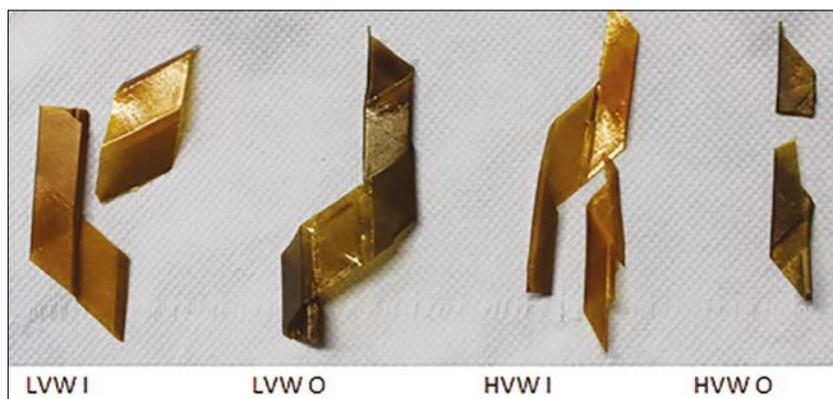
Figure 9. Paper samples of a real transformer, which was in operation for more than 50 years.
