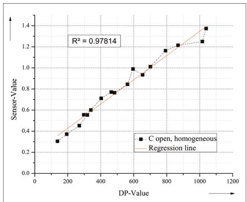
Figure 7. Linear correlation between the sensor-value and the DP-value for Oil C in an open system with a homogeneous arrangement
