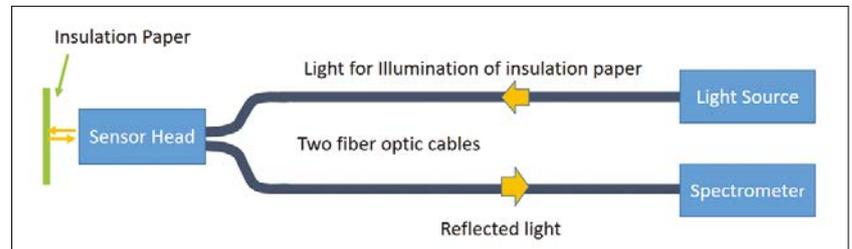
Figure 3. Principle of optical reflection spectroscopy of insulation paper
