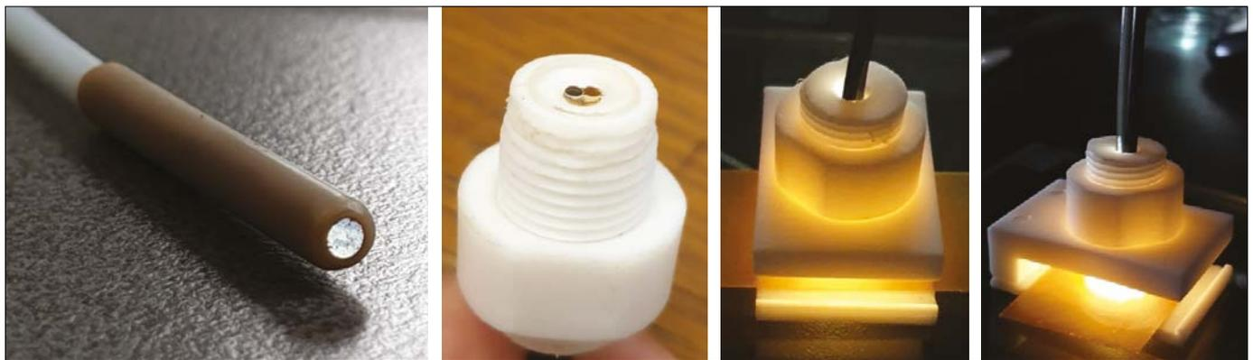
Figure 10. Sensor heads for use in transformer (two left), two right: with a holder for insulation paper
