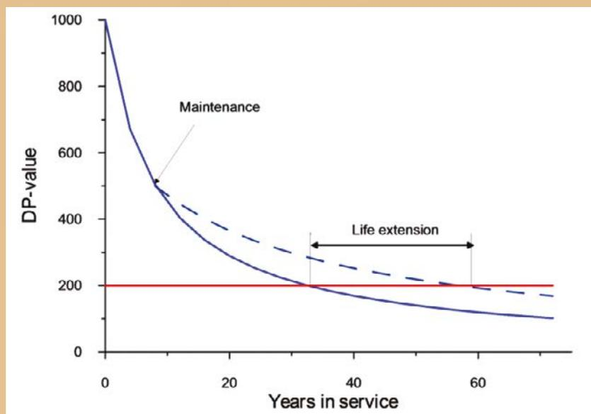
Figure 1. Online monitoring of DP-value for proactive lifetime and maintenance management [6]
