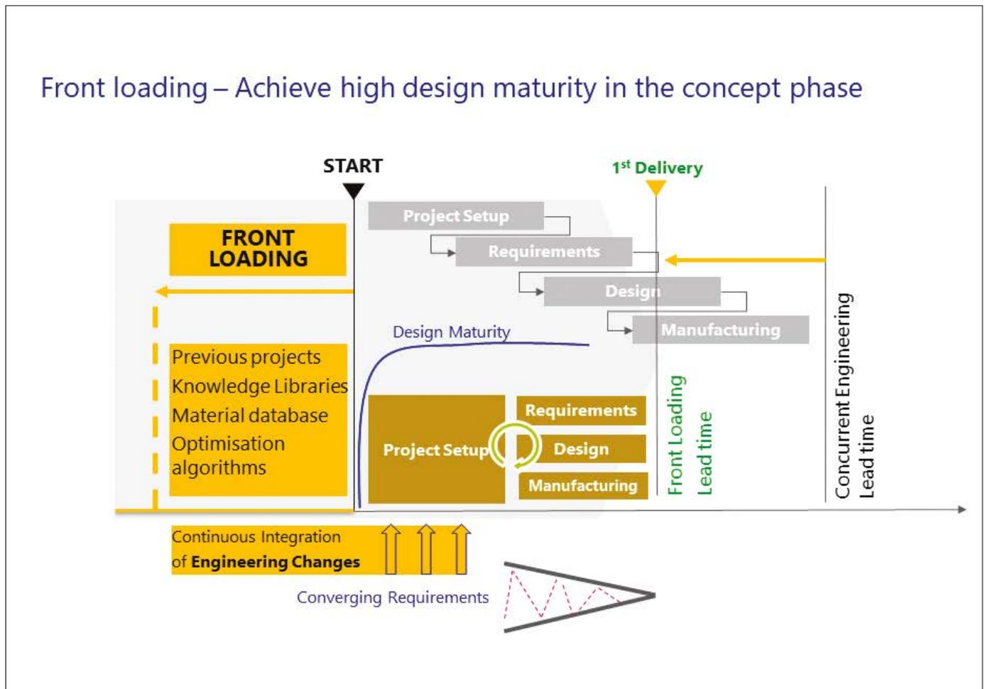
Figure 4. Innovative front-loaded design process to achieve a high level of design maturity in the initial phase itself. This can significantly reduce design lead time compared to concurrent engineering.
