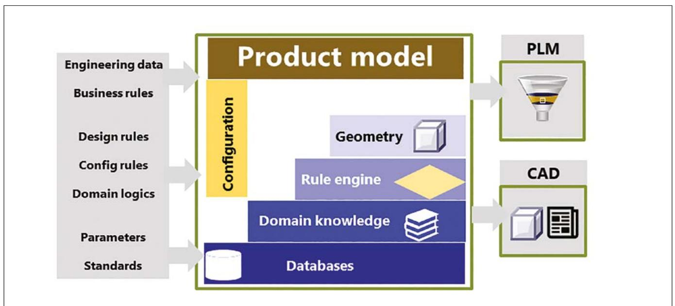
Figure 3a. Architecture and sub-modules in developing a product model – the nucleus of a knowledge-based engineering system
