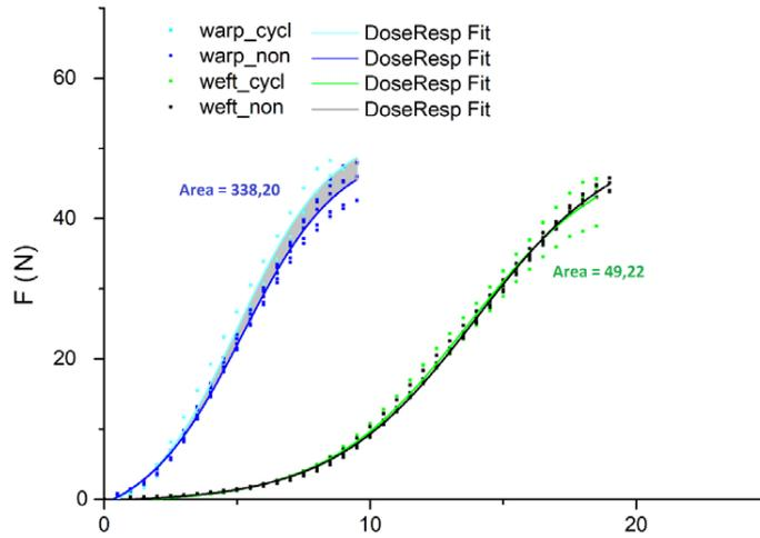
Figure 3. Tensile behaviour of the basket weave fabric before and after cyclic loading
