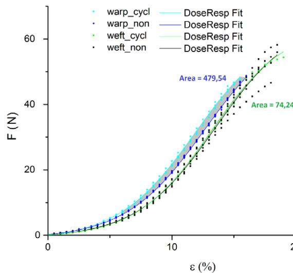
Figure 2. Tensile behaviour of the plain weave fabric before and after cyclic loading; where: warp\_cycl – warp direction after cyclic loading, warp\_non - warp direction before cyclic loading, weft\_cycl – weft direction after cyclic loading, weft\_non – weft direction before cyclic loading
