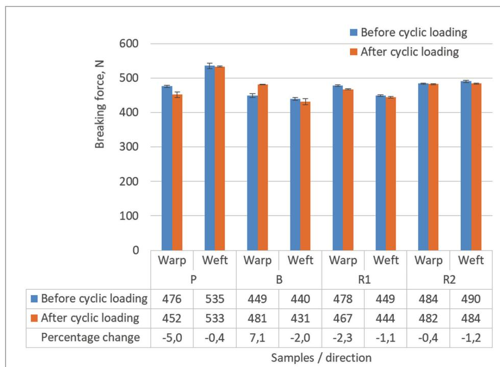
Figure 6. Breaking forces of the fabrics before and after cyclic loading with error intervals
