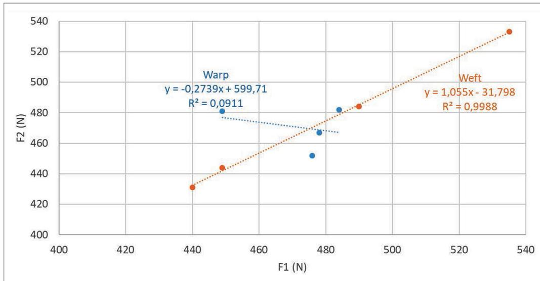
Figure 7. Regression lines and regression coefficients for the forces at break before and after cyclic loading; F1 – breaking forces before cyclic loading (N), F2 – breaking forces after cyclic loading (N)
