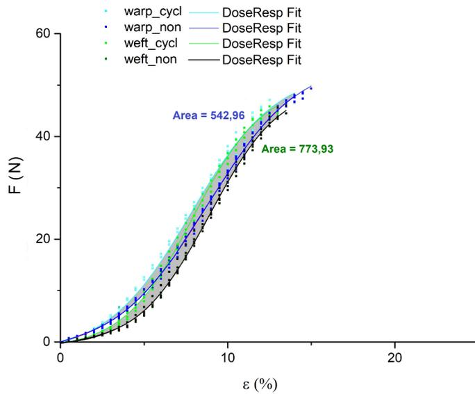
Figure 4. Tensile behaviour of the longitudinal rib weave fabric (R1) before and after cyclic loading
