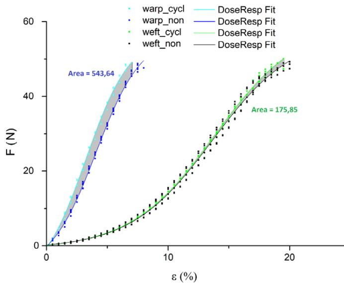
Figure 5. Tensile behaviour of the transversal rib weave fabric (R2) before and after cyclic loading
