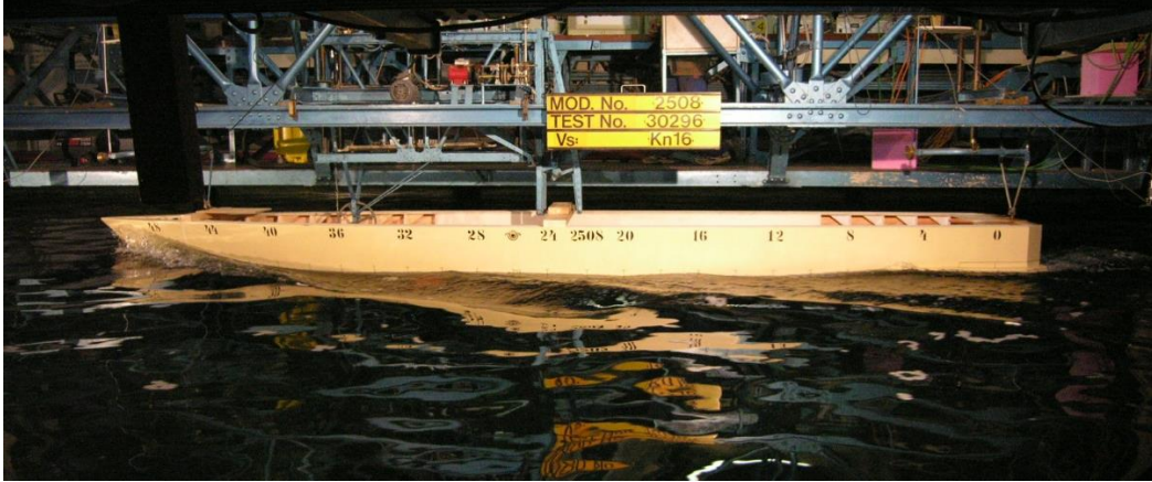
Fig. 3 Model test setup for resistance test [24]
