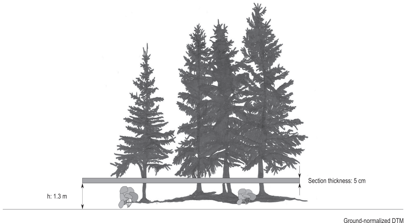
Fig. 4 Visualization of data slicing for generating cross-sections
