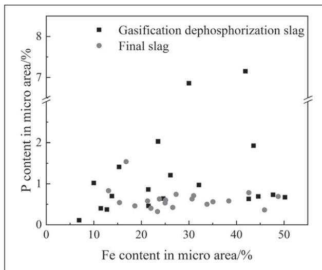
Figure 6 P and Fe in RO phase of final slag and Fe phase of phosphorus vaporization slag
