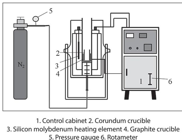
**Figure 1** Equipment schematic diagram
