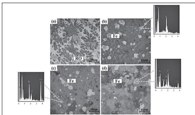
Figure 5 SEM-EDS analysis of slag samples
