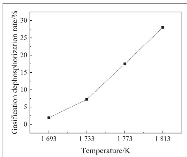
**Figure 2** Effect of temperature on the gasification dephosphorization rate
