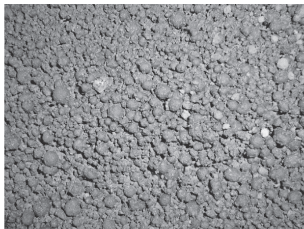
Figure 2 Sample of zinc-bearing feedstock after the pelletisation procedure.
