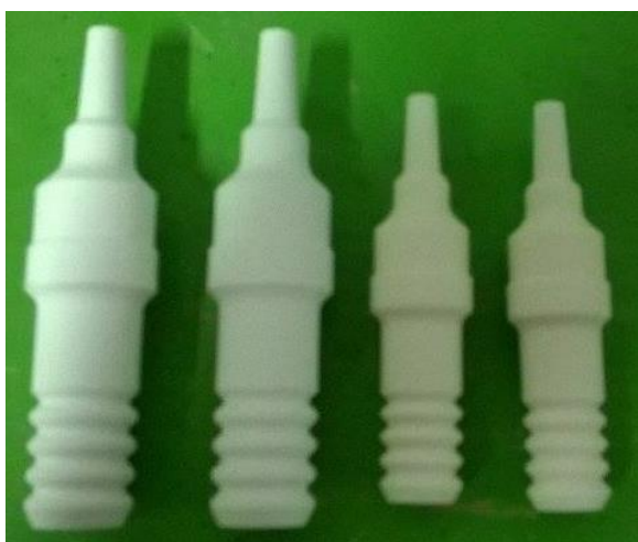
Figure 2. Ceramic part of the car spark plug (before and after sintering)
