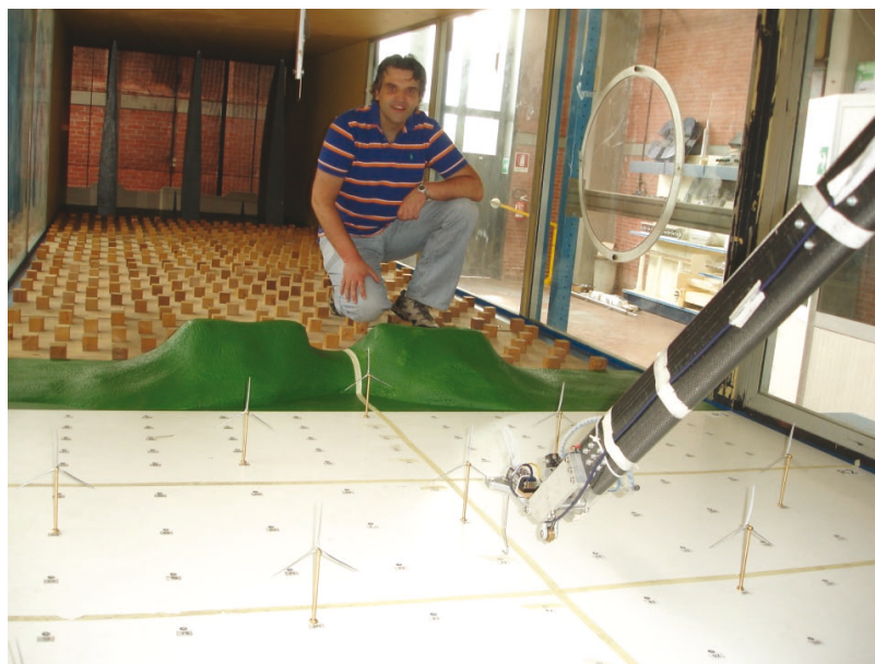
Hrvoje Kozmar in the test section of a boundary layer wind tunnel at the University of Florence, Italy -- model experiments on wind characteristics in wind farms situated on a hilly terrain
