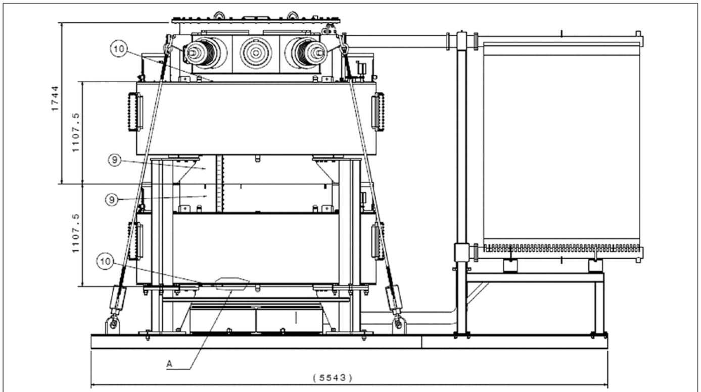
Figure 6. GA of 36 kV FCL reactor tank, radiators and SC magnets
