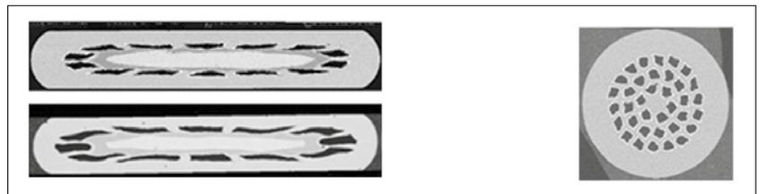
Figure 5: Cross-section of multifilamentary  $MgB_2$  tapes and wires ( $MgB_2$  filaments in black)
