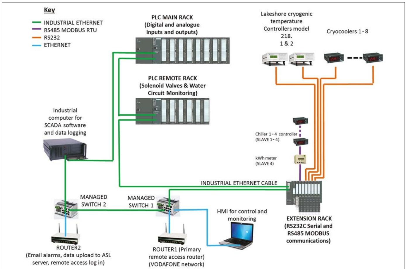
Figure 12. FCL control and SCADA systems
