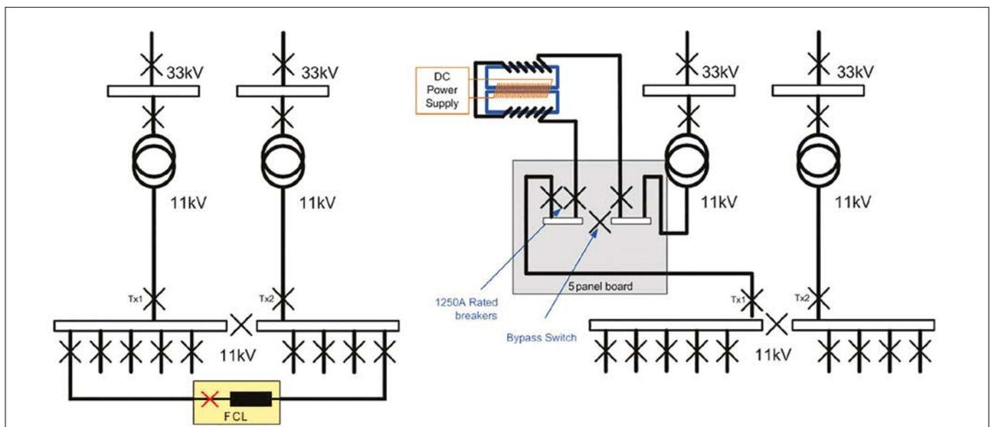
Figure 14. Bus-section (left) and transformer tail (right) FCL deployments
