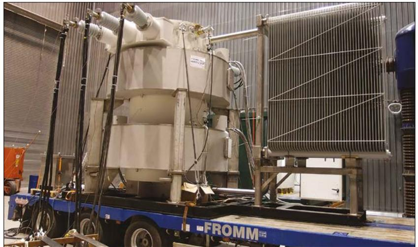
Figure 8. FCL during Thermal Test at IPH, Berlin
