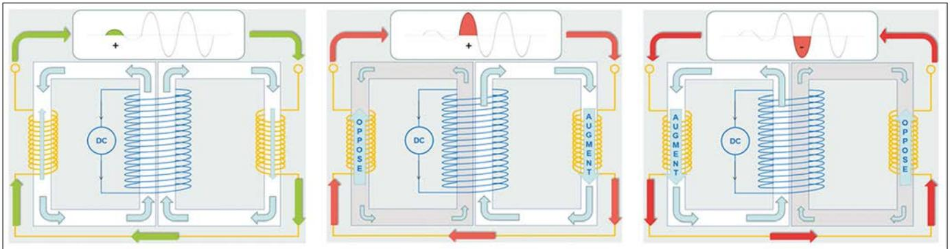
Figure 2. Closed-core arrangement (left) under load current (centre and right) during a fault
