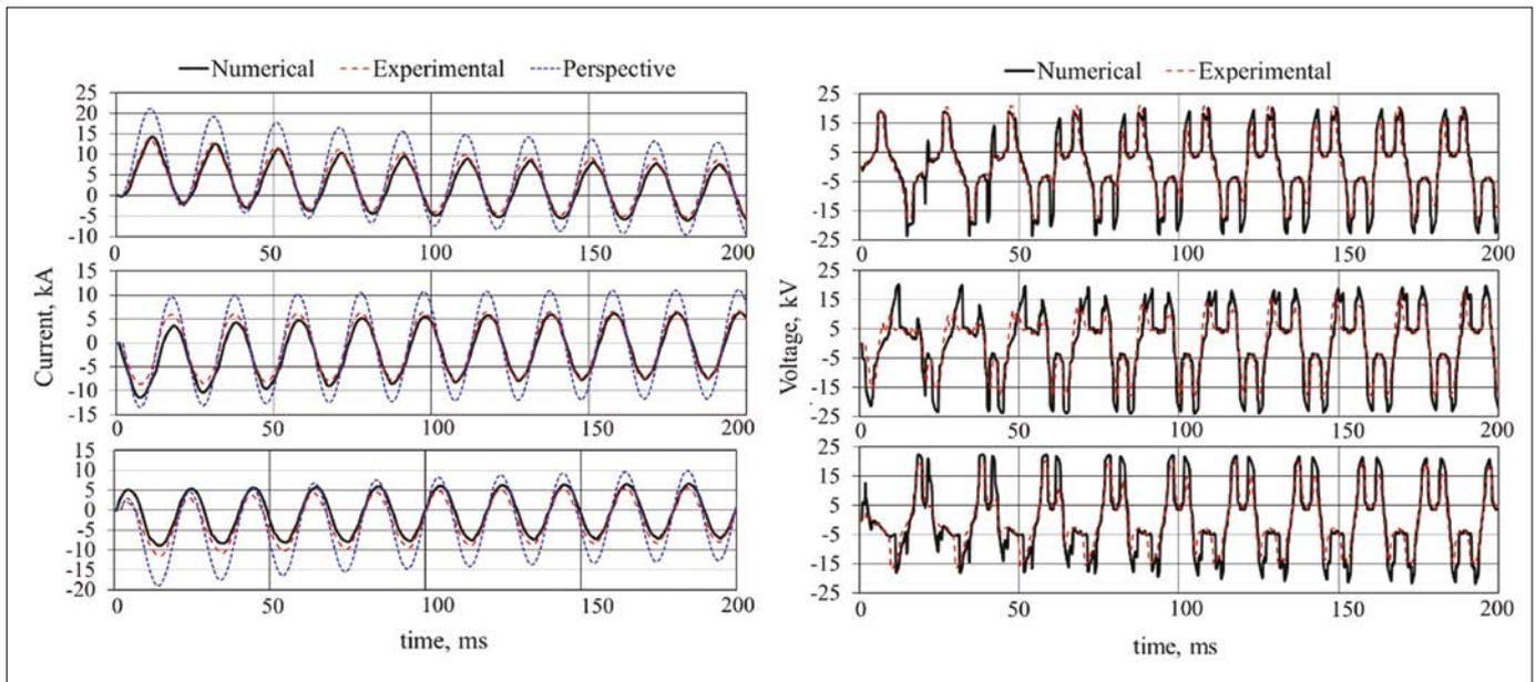
Figure 15. Results of short-circuit tests showing prospective and limited (measured and calculated) currents (left) and (measured and calculated) voltage drops across the device (right)
