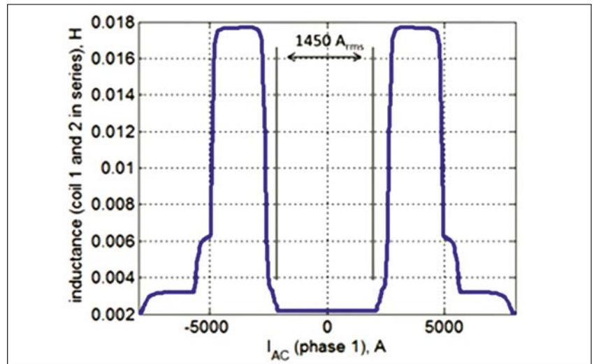
Figure 7. FCL AC coils inductance vs AC current
