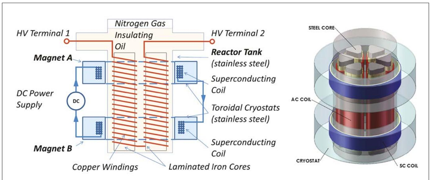
Figure 3. Open-core arrangement showing active parts of one phase (left) and 3 phases (right)
