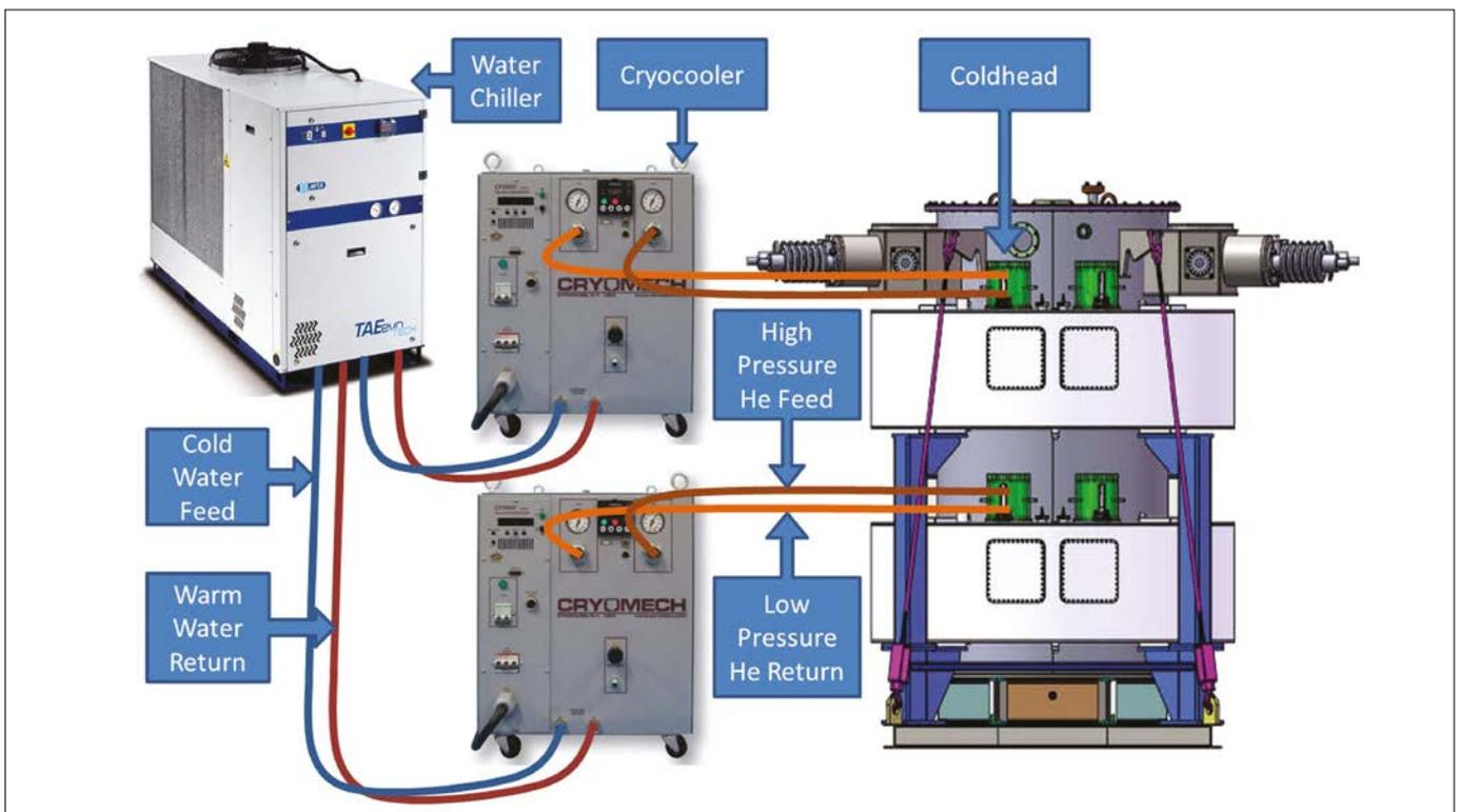
Figure 11. Schematic layout of the FCL magnets cooling system
