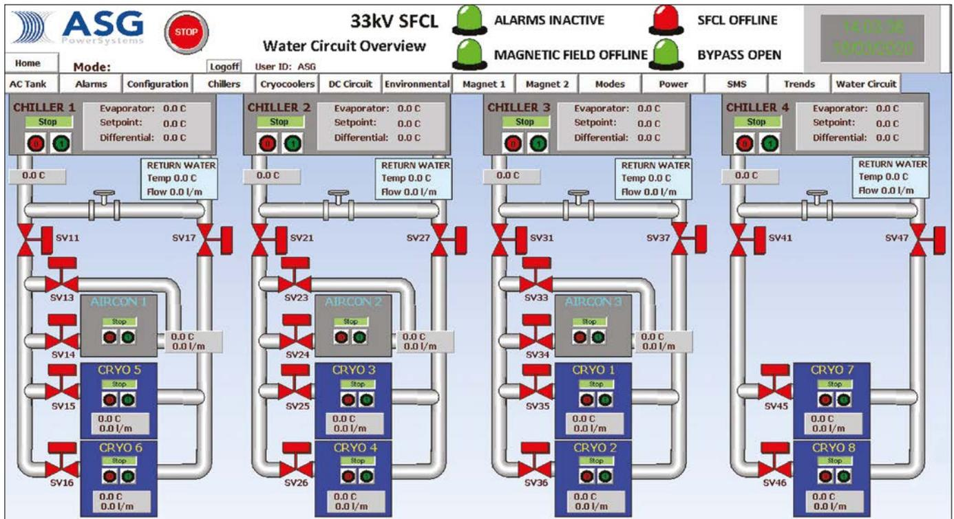
Figure 13. Cooling water system SCADA screen
