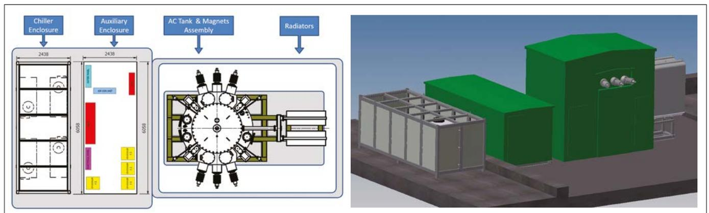
Figure 9. Typical layout of the three FCL enclosures
