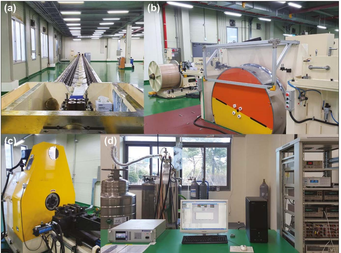
Figure 1. Our facilities for commercial-scale wire production and measurement: (a) a 25 m linear drawbench; (b) a bull block equipped with a 1.5 m diameter capstan drum; (c) a 20-horsepower rotary swaging machine; (d) measurement systems for electromagnetic properties of superconducting wires.
