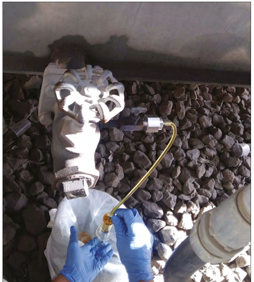
Figure 9. One valve to ports, which is the correct one for oil sampling?
