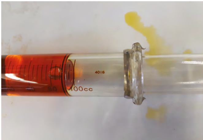
Figure 13. A leaking syringe (left) versus one sealed with special grease (True North by Morgan Schaffer)
