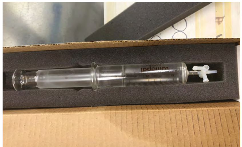
Figure 12. A special box for preserving sensitive syringes during transportation
