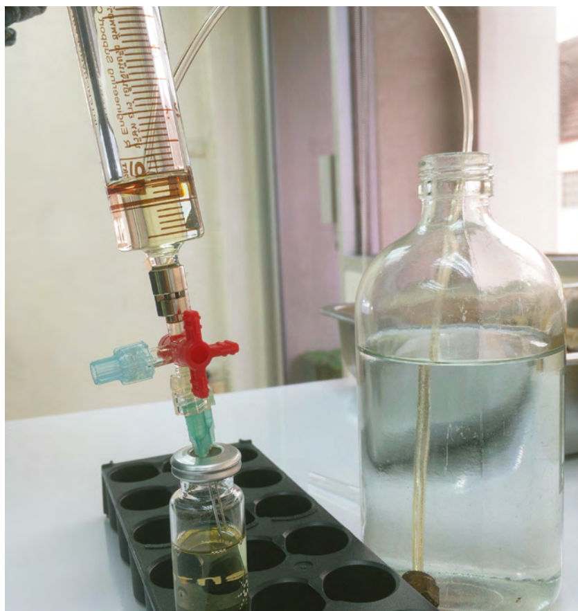
Figure 11. Direct transfer of the oil to the vial for being tested according to headspace DGA
