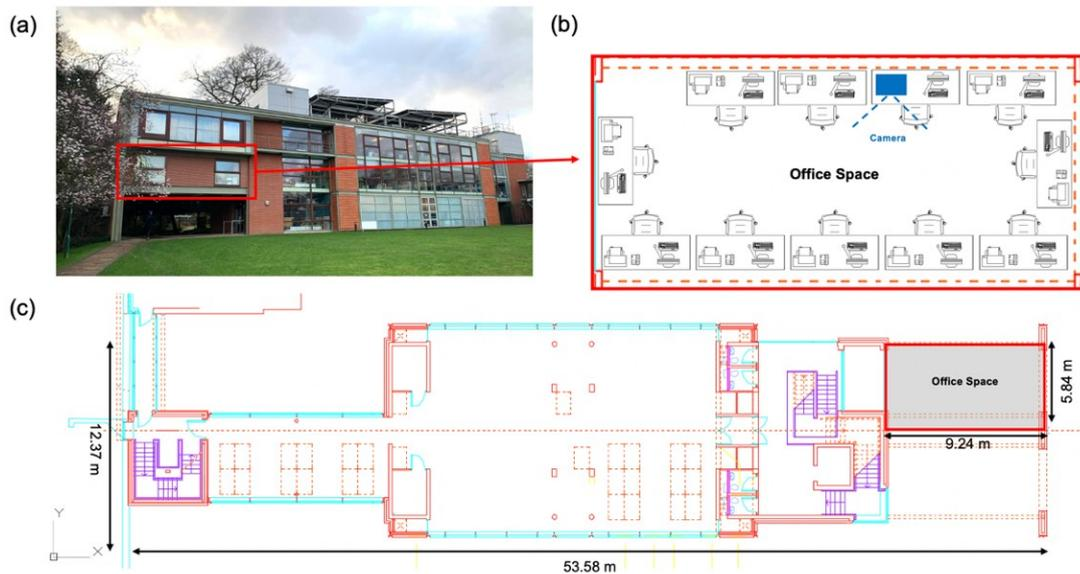
Figure 5. Sustainable Research Building at University Park Campus, University of Nottingham, UK: photo (a); experimental set up (b); 1st floor plan (c)
