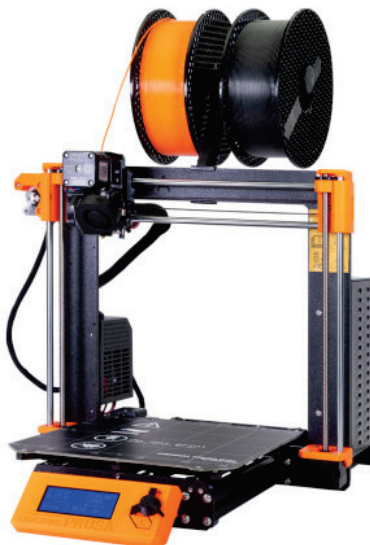
Figure 6 FFF machine Prusa i3 MK3S
