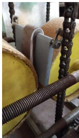
Figure 3. The process of implementing a five-layer squeezing of semi-finished wet leather products
