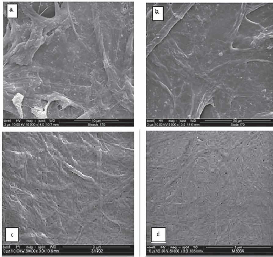
**Figure 6** FE-SEM micrographs of a) soda pulp sheet, b) MEA pulp sheet, c) soda-NFLC films and d) MEA-NFLC films
