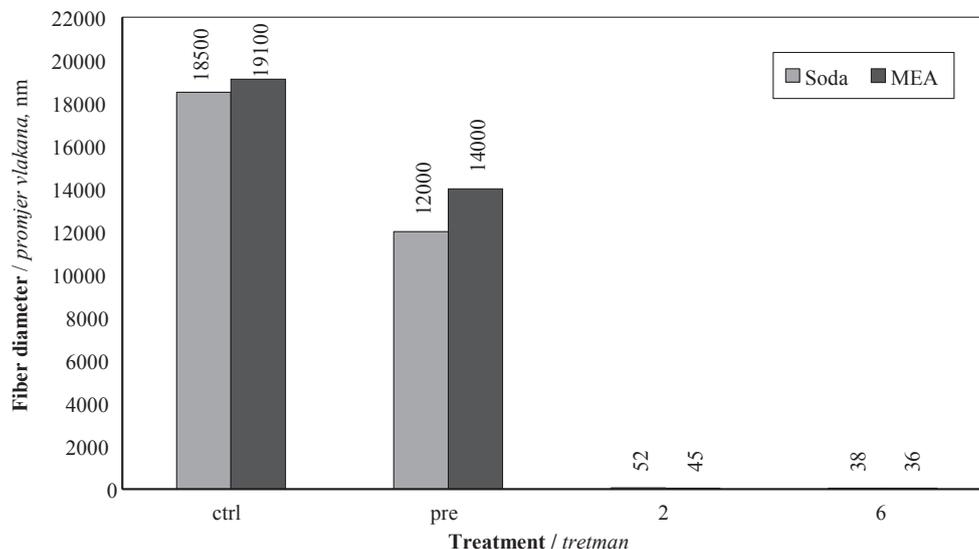
**Figure 7** Fibers diameter of NFC films from soda and MEA pulps
