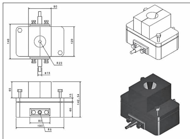
Figure 1 Dimensions and 3D view of the steel mold
