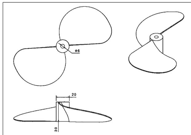
Figure 2 Dimensions of the ship's propeller
