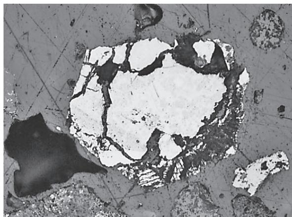
**Figure 5** Grain of bixbyite in a relic with braunite and in the intergrowth of a nonmetallic mass, magnification is 200
