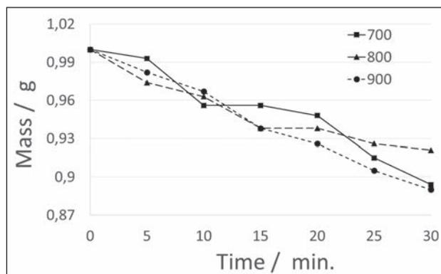
Figure 4 Changes in sample weight during the roasting of zinc sulphide in a horizontal tube furnace
