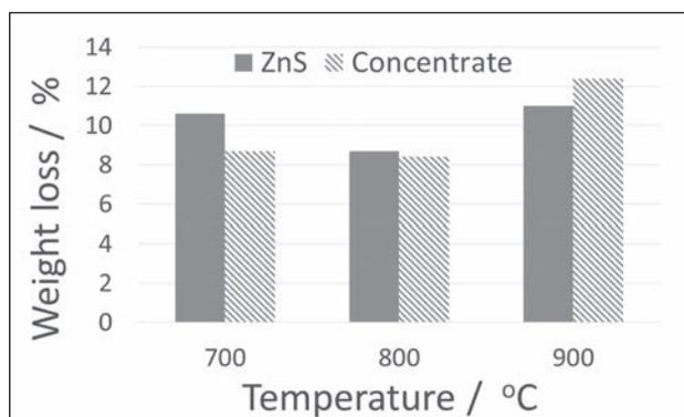
Figure 6 Weight loss of ZnS samples and zinc sulphide concentrate after 30 minutes of roasting in a horizontal tube furnace
