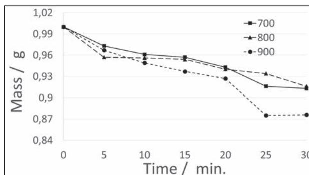
Figure 5 Changes in sample weight during the roasting of sulphide zinc concentrate in a horizontal tube furnace
