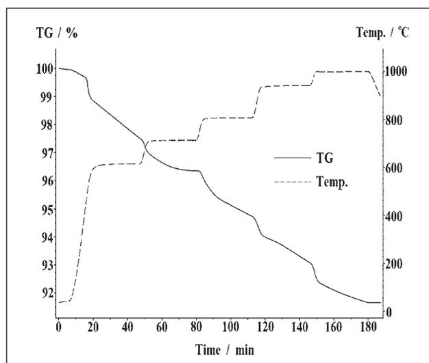
Figure 3 TG curve for zinc sulphide concentrate
