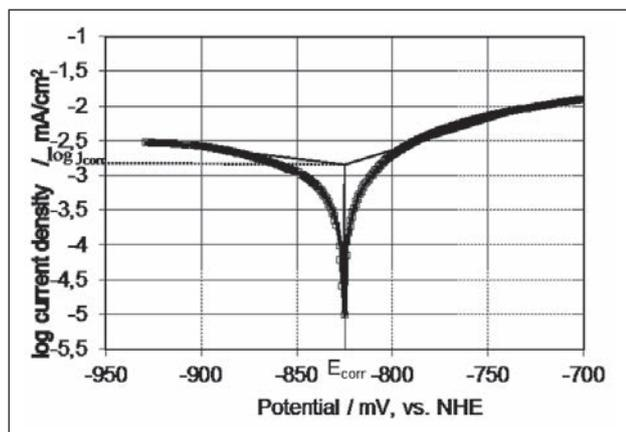
**Figure 2** Curves of anodic and cathodic polarization of Zn-5Al coating in 3,5 % NaCl solution
