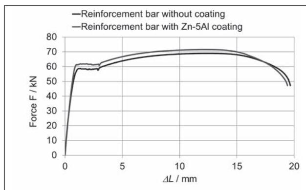
**Figure 3** Tensile diagrams for reinforcement bar without coating and with Zn-5Al coating
