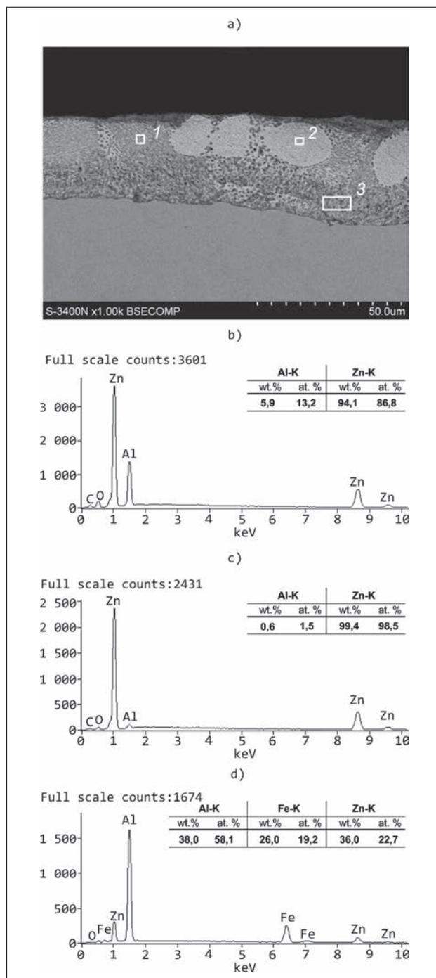
**Figure 1** Microstructure of the Zn-5Al coating on reinforcement steel (a) and results of EDS microanalysis in the diffusion layer of the coating
