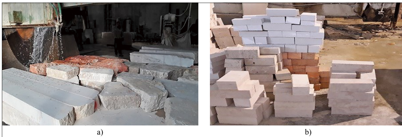
Figure 2: Rock sampling procedure: a) cutting of rock samples; b) preparation of samples for transferring to laboratory
