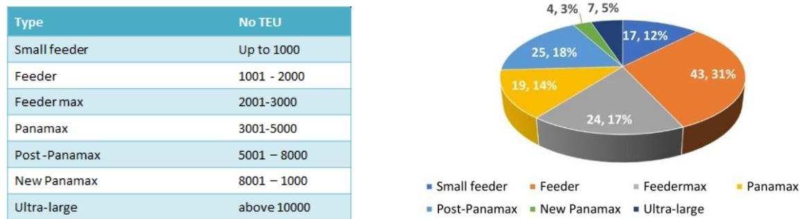
**Fig. 5.** Container ship types (left) and distribution of container ships by type visiting Black Sea ports (right)
