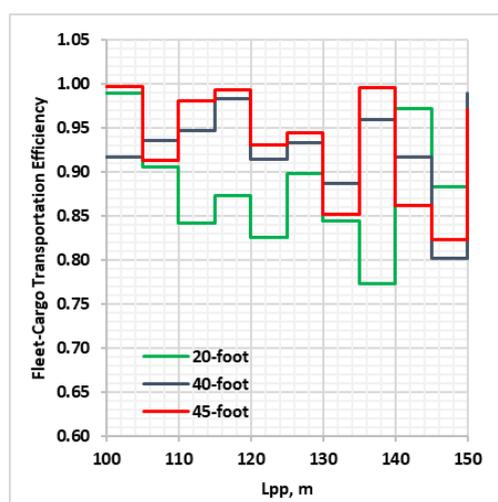
**Fig. 12.** Fleet-cargo transportation efficiency,  $\psi=1$
