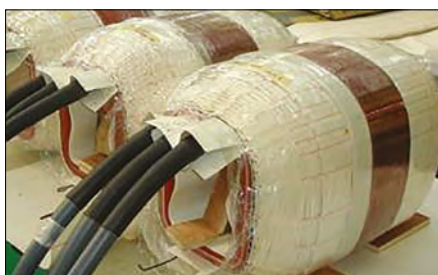
Figure 1. HV and LV coils
