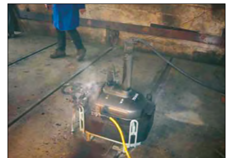
Figure 6. SIDT after destructive short circuit test
