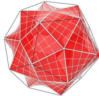
Figure 11: The dodecahedron's faces are completely replaced by paraboloid patches.
