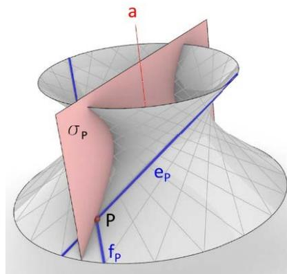
Figure 5: One symmetry plane of two intersecting generators of an R-hyperboloid  $\Phi_R$  contains the axis  $a$  of  $\Phi_R$ .
