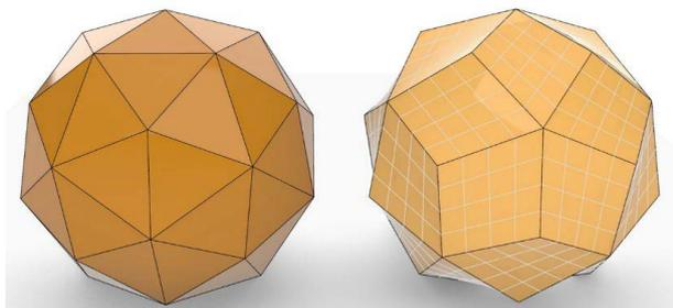
Figure 12: The dodecahedron’s faces are completely replaced by paraboloid patches.
