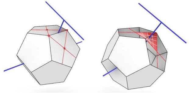
Figure 10: The principle, how one can proceed in case of non-triangular faces of a polyhedron, shown at a regular dodecahedron
