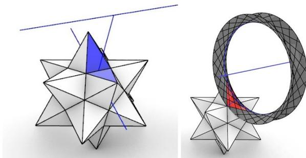
Figure 13: A Kepler star with an R-hyperboloid patch through an equilateral edge quadrilateral
