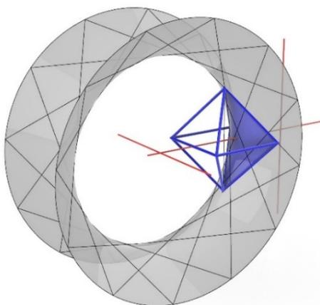
Figure 3: R-hyperboloid  $\Phi_{R2}$  through an edge-quadrilateral of an octahedron
