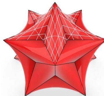
Figure 14: A Kepler star completely covered with R-hyperboloid patches
