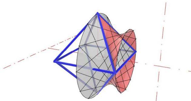
Figure 4: R-hyperboloid  $\Phi_{R3}$  through an edge-quadrilateral of an octahedron
