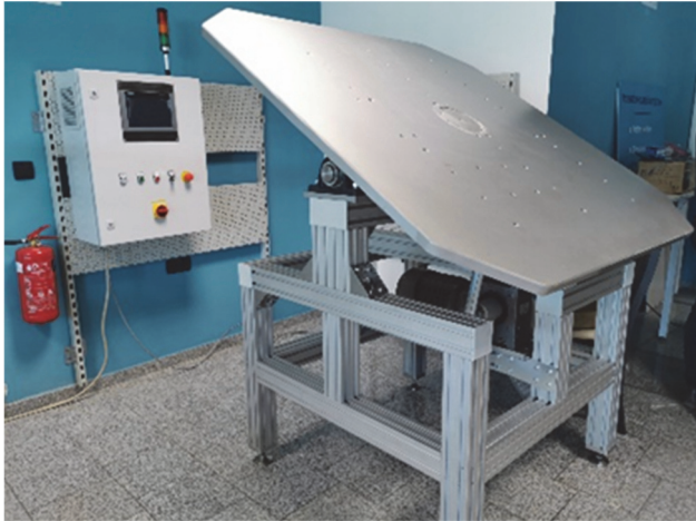
Figure 6 Test rig for oscillation simulation layout
