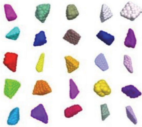
Figure 5 Simulation model of ballast
