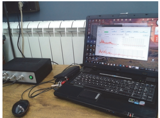
Figure 3 VibroLog measuring system
