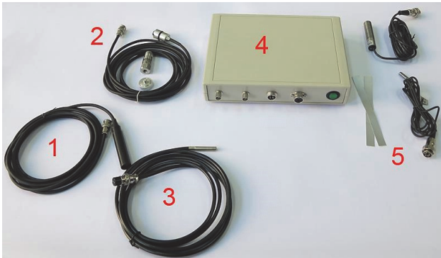
Figure 1 VibroLog measuring system with sensors
