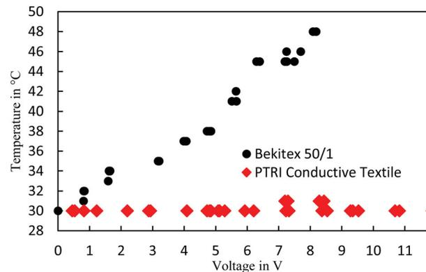
**Figure 5.** Voltage vs Temperature response of BK 50/1 and PTRI conductive textile.
