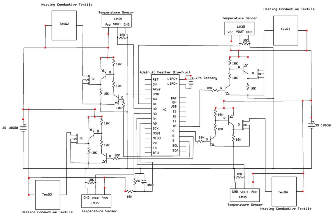
Figure 3. E-textile belt schematic diagram.
