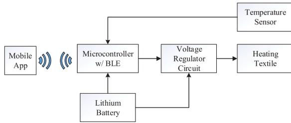
Figure 2. E-textile heating system framework.
