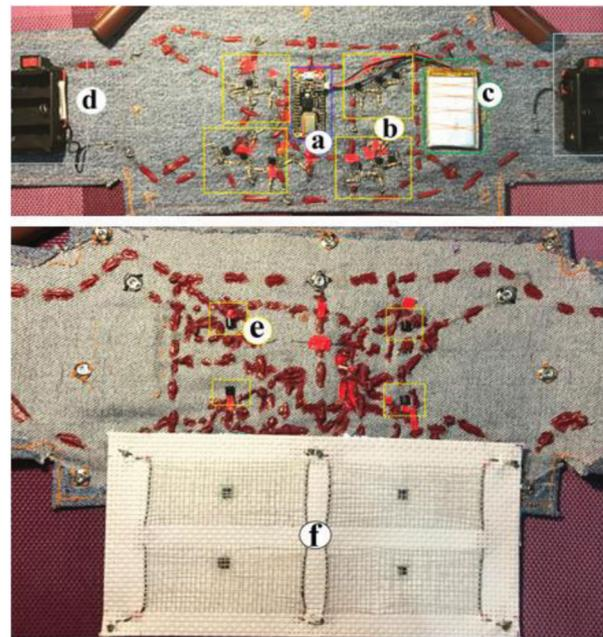
**Figure 1.** Wireless heating e-textile belt parts: (a) Adafruit Feather 32u4 Bluefruit LE, (b) Voltage Regulator Circuit, (c) LiPo Battery, (d) 18650 Batter Pack, (e) Temperature Sensor, (f) 4-quadrant Heating Textile.
