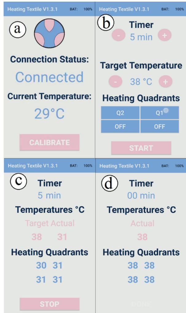
**Figure 4.** Android application user interface pages: (a) Calibrate Page, (b) Start Page, (c) HeatUp Page, and (d) Done Page.
