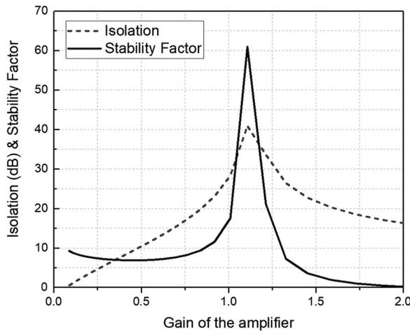
**Figure 5.** Stability factor and isolation of the proposed isolator as functions of the voltage gain of the amplifier.
