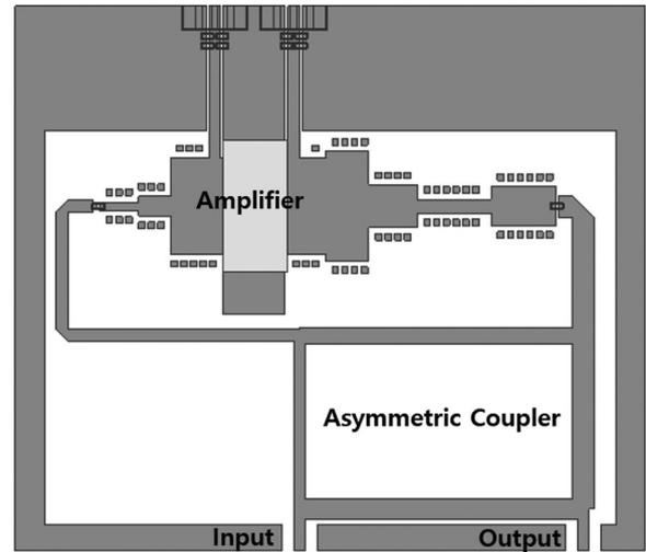
**Figure 3.** Layout design of the 2.45 GHz isolator on an FR4 printed circuit board.
