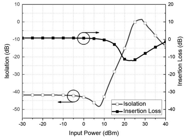
**Figure 6.** Performances of the 2.45 GHz isolator in large-signal simulation.
