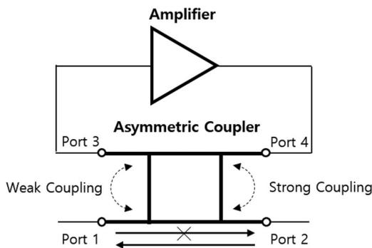
**Figure 1.** Block diagram of the proposed isolator based on an asymmetric coupler.
