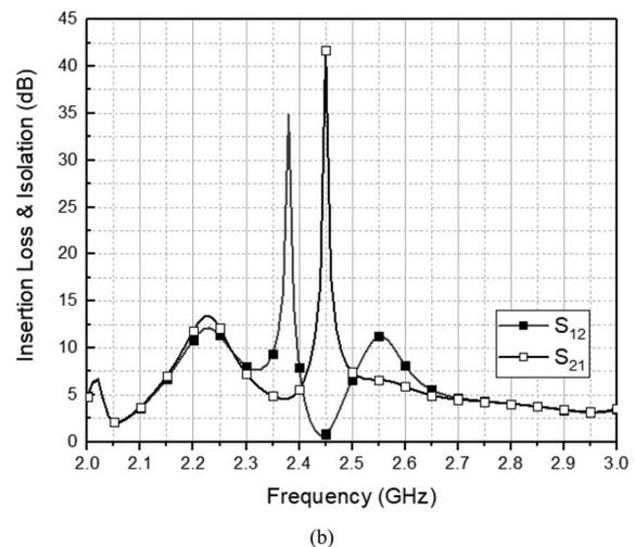
**Figure 4.** EM-circuit co-simulation results for the proposed isolator: (a) Input ( $|S_{11}|$ ) and output ( $|S_{22}|$ ) return losses; (b) Insertion loss ( $|S_{12}|$ ) and isolation ( $|S_{21}|$ ).
