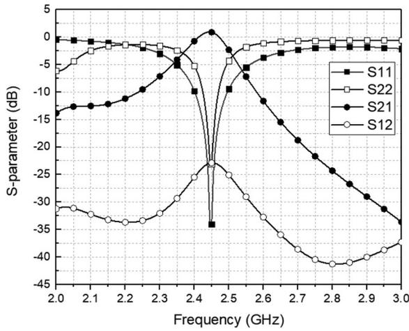
**Figure 2.** Simulated S-parameters of the amplifier itself in the proposed isolator.
