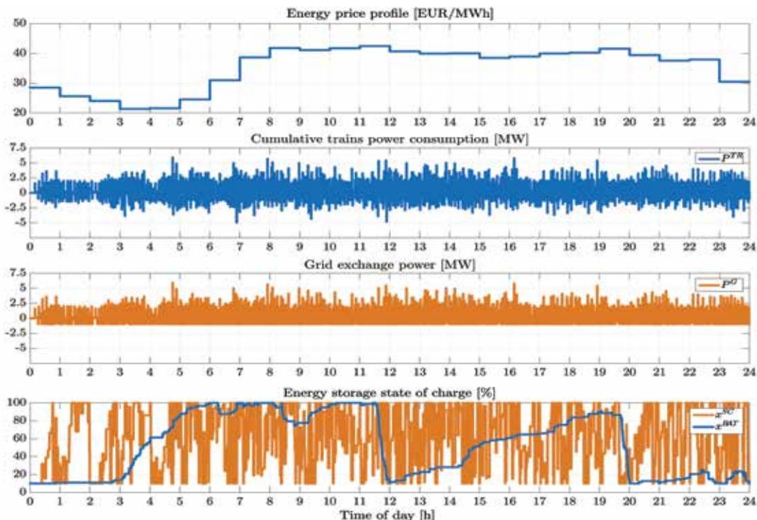
**Fig. 4.** Daily power flows for system operation with only higher level MPC installed and grid receptiveness of -1 MW
