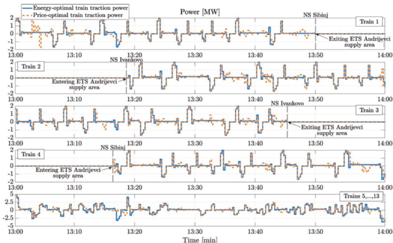
Fig. 7. Power consumption profiles of all trains supplied from ETS Andrijevci, before and after hierarchical coordination, for a one-hour system operation
