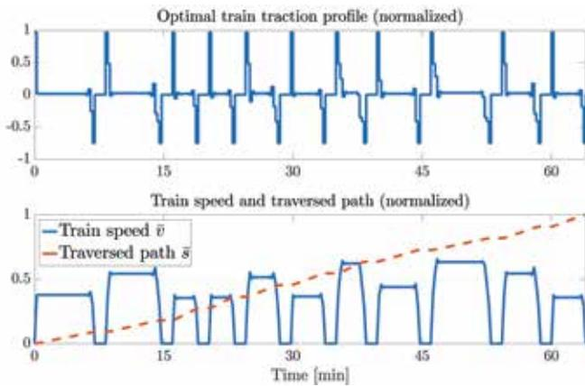
**Fig. 3.** Energy-optimal train traction force, speed and traversed path profiles while traveling from Slobodnica to Ivankovo.
