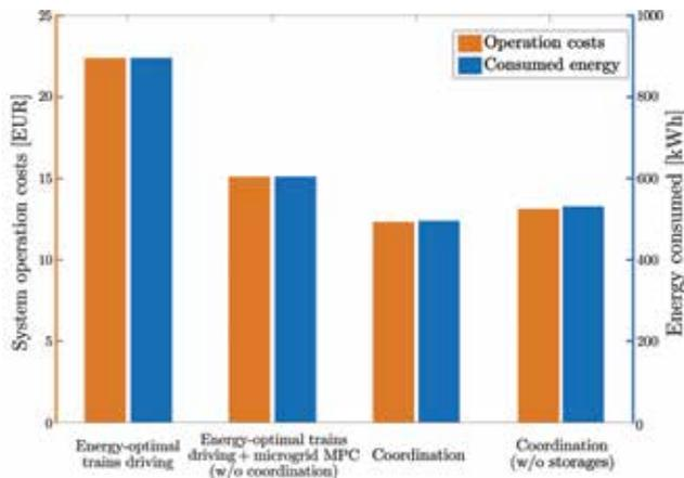
**Fig. 8.** Energy consumption and system operation costs for different control setups for the one-hour system operation
