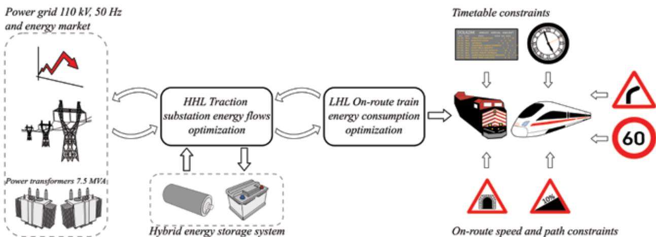
Fig. 1. Scheme and information flow of hierarchical coordination between LHL and HHL optimizations.
