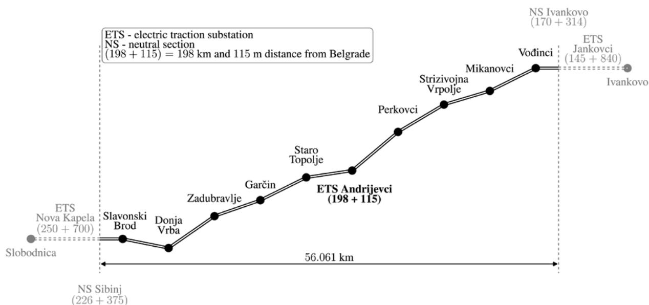
Fig. 2. Croatian Railways Corridor X section area supplied from ETS Andrijevcı with the corresponding passenger stations.
