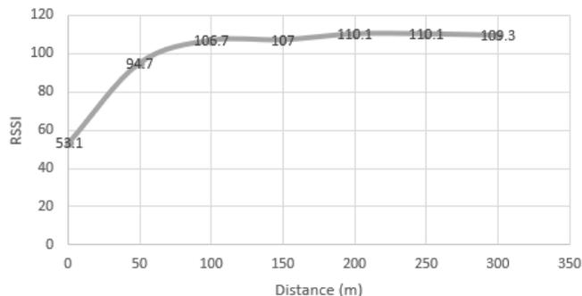
Fig. 9. Receiver Signal Strength Indicator (RSSI) Testing Result
