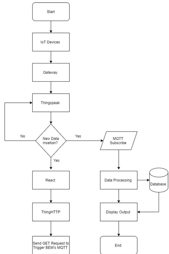
Fig. 2. Proposed flowchart of the data flow
