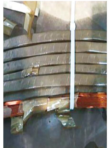
Figure 5. Bunched conductor (inter conductor) fault [12]
