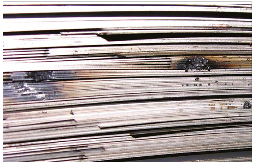
Figure 3. The so-called “fire in steel” (Source: Ibragim Murataev, Russia)
