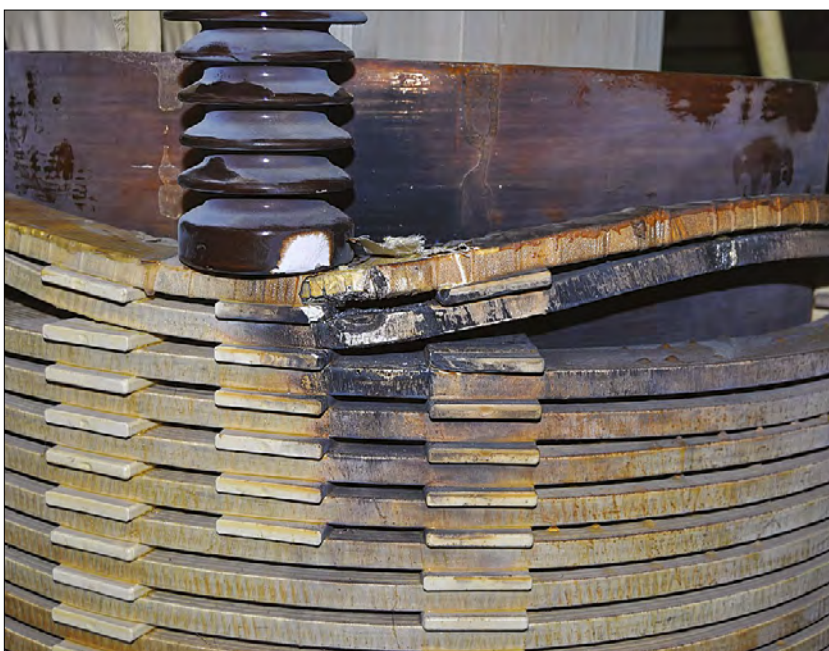
Figure 2. Damage due to short circuit between the winding discs (Source: http://www.nov-electro.com/2013/foto-transformator-plant )
