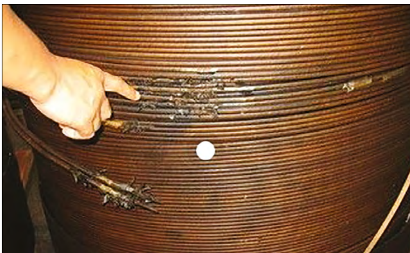
Figure 1. Shorted turn-to-turn (Source: testguy.net)
