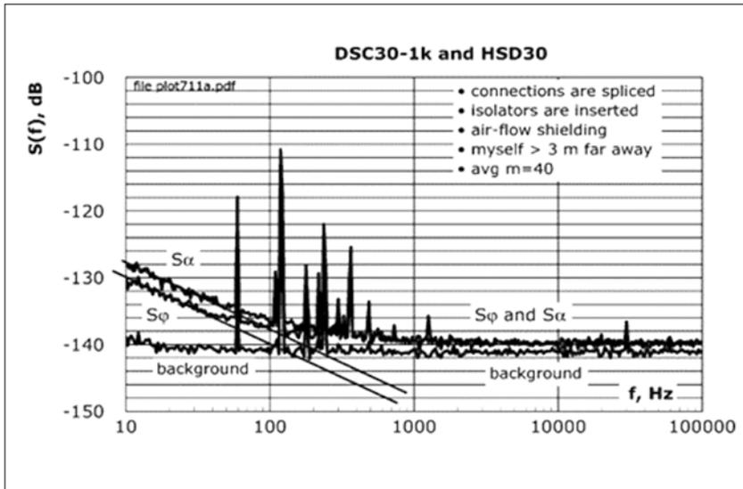
Figure 7. A typical amplitude spectrum of the flicker noise [12]
