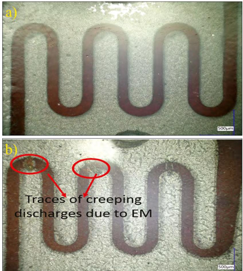
Figure 26. The magnified substrate of two photoresistors: a) an unused photo resistor b) after subjecting to some arcs
