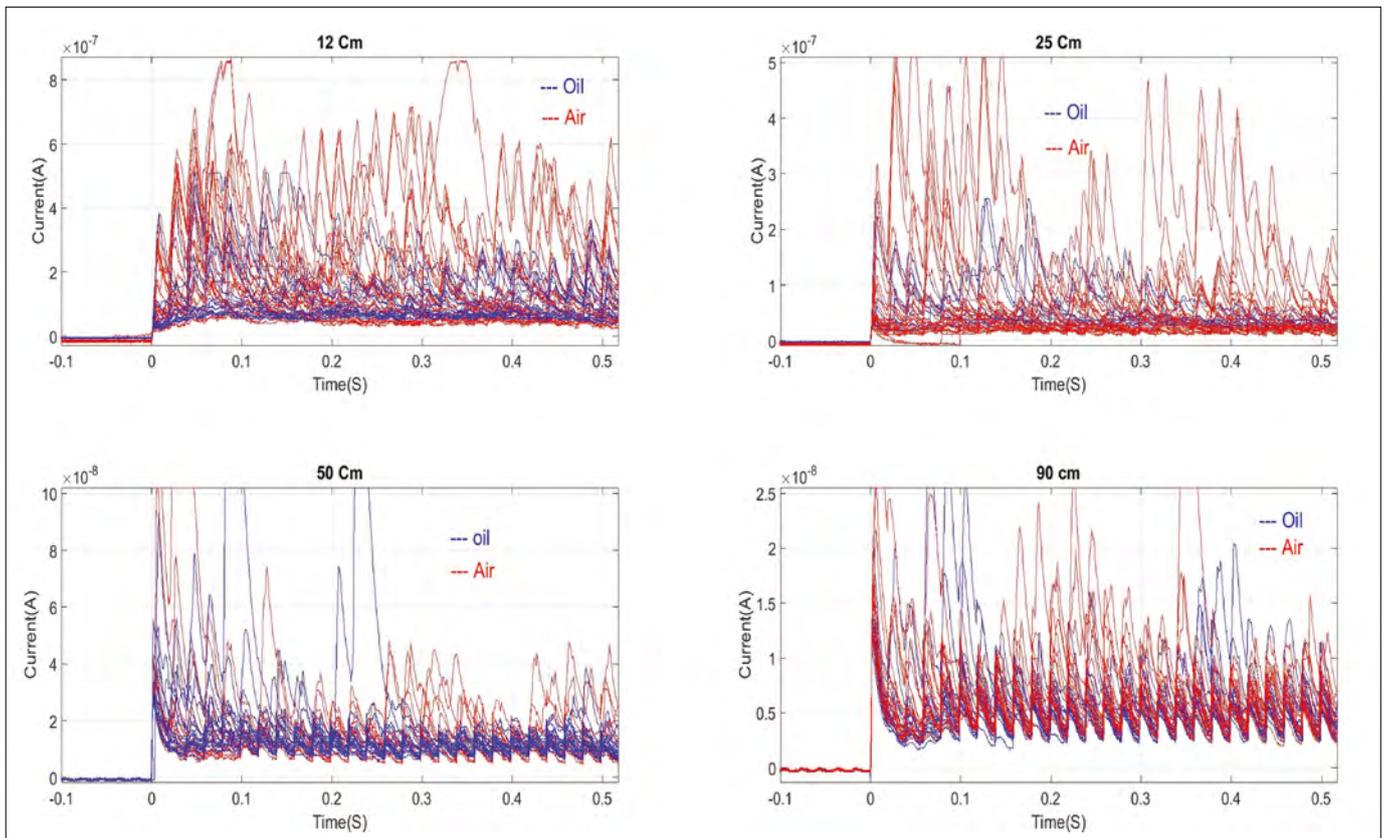
Figure 14. Comparison of the measured current in oil and air for a high number of arcs
