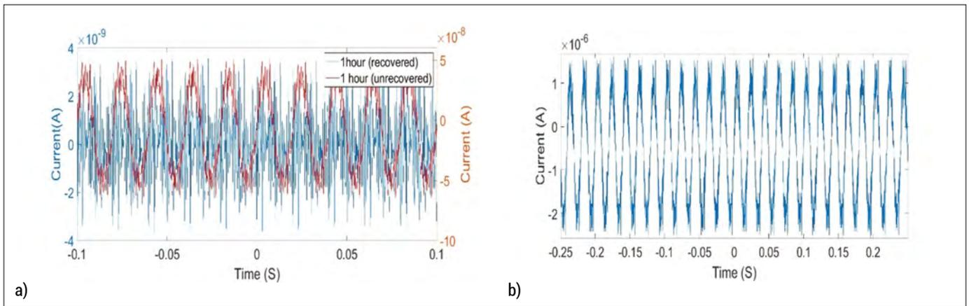
Figure 21. a) Comparison of dark current in recovered and unrecovered sensors. b) A dramatic increment of the dark current as for a typical sensor
