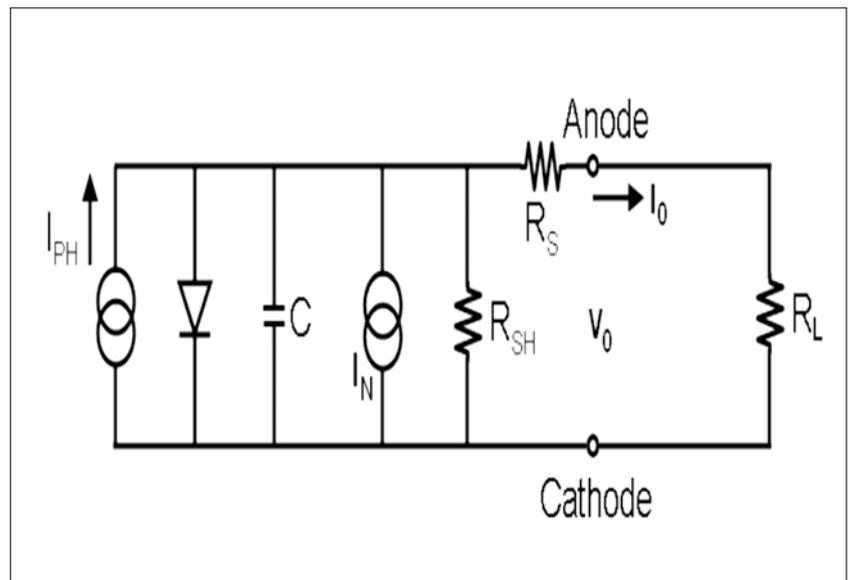
Figure 6. An electrical model for photodiodes [10]
