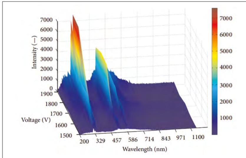
Figure 2. The light intensity of a 50 Hz electric arc at different voltage-wavelength [7]
