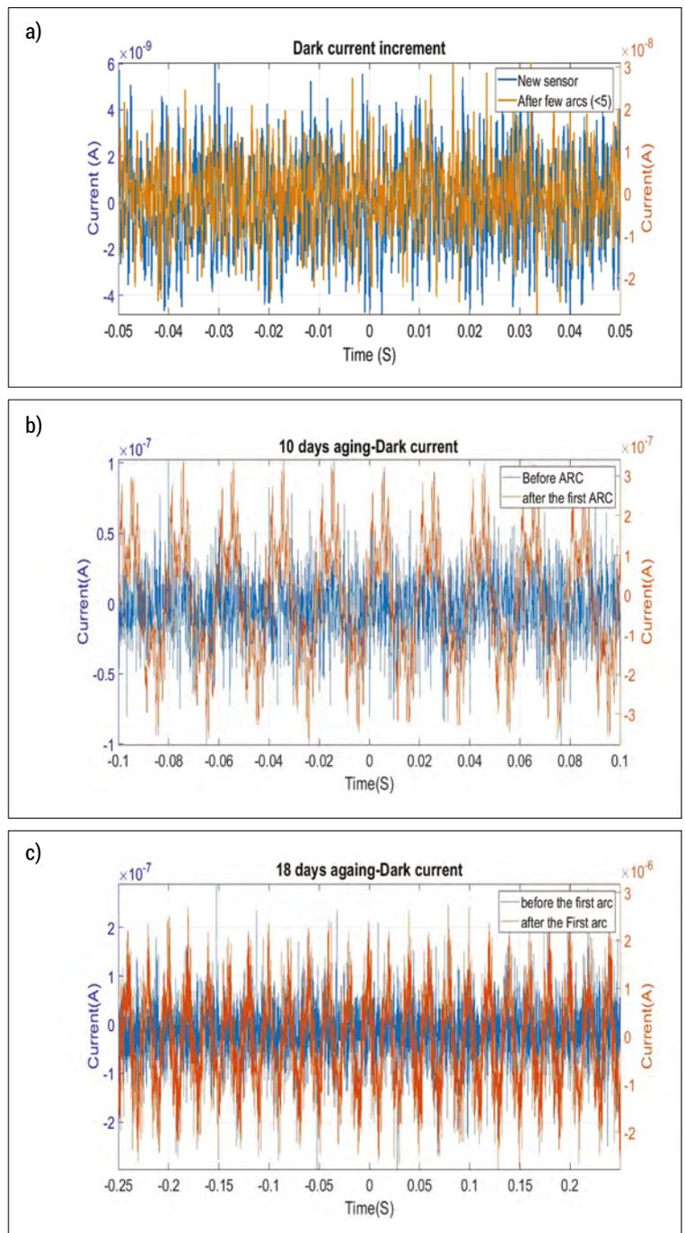
Figure 22. The effect of thermal ageing in oil on the amount of dark current: a) unused sensor b) after ten days ageing c) after 18 days ageing
