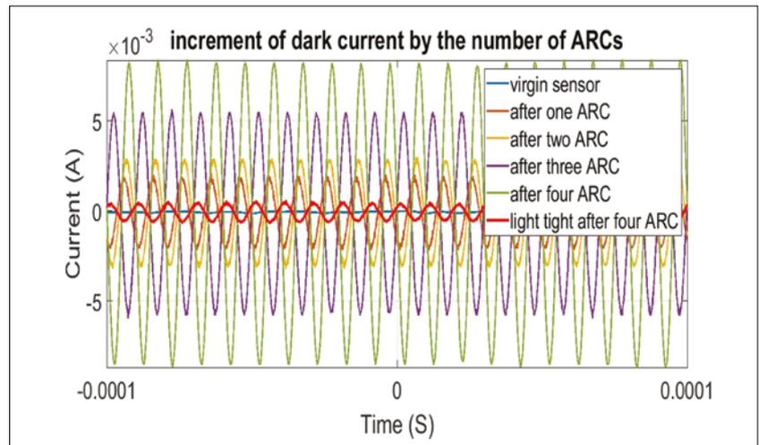
Figure 25. Increment of the dark current after each arc for the photoresistors
