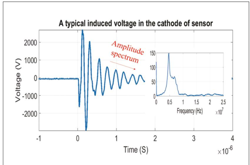
Figure 4. Potential of the cathode in a photodiode adjacent (12 cm) to a 50 Hz electric arc at the time of arc formation
