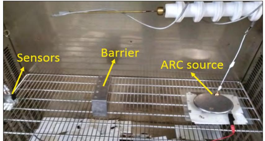
Figure 17. A typical configuration for the barrier effect
