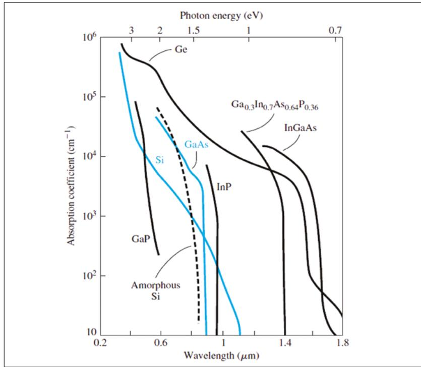
Figure 1. The absorption coefficient of some materials with respect to the wavelength and photon energy [3]
