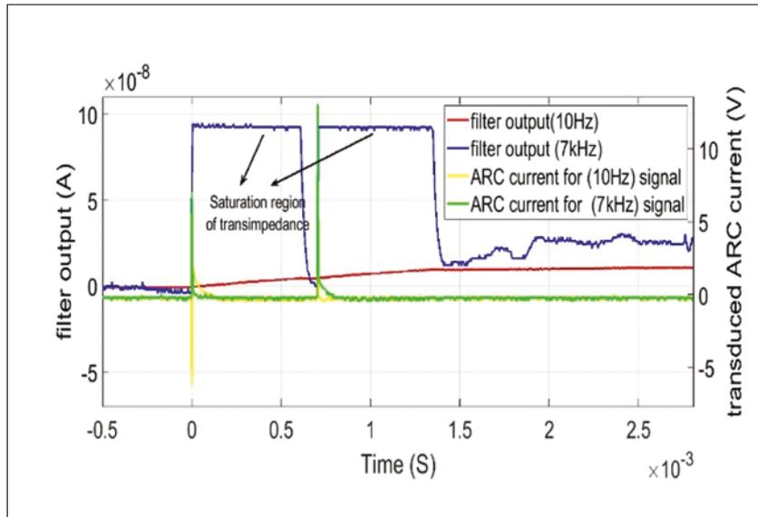
Figure 11. The effect of filtering on the output signal
