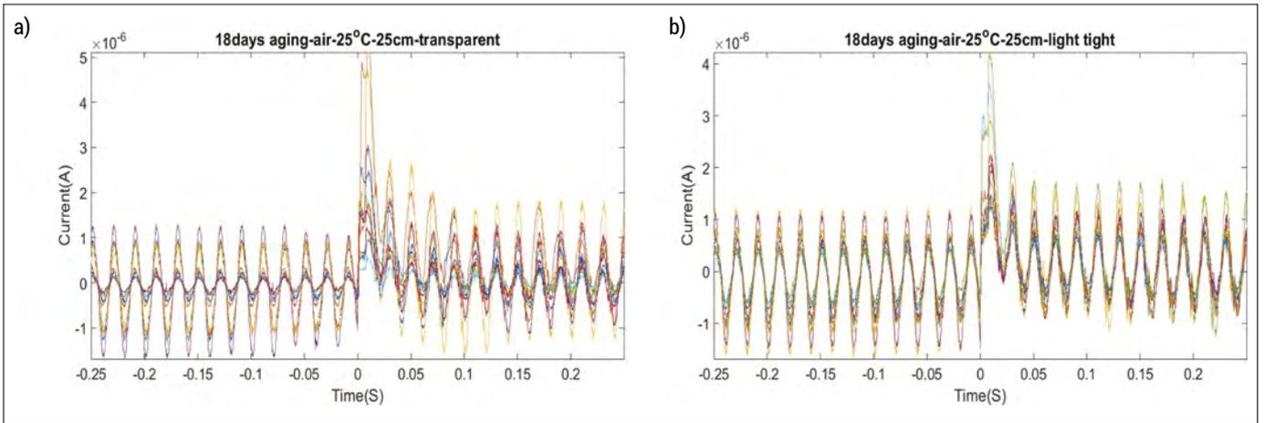
Figure 23. a) the output signals for a transparent sensor after 18 days ageing, b) corresponding signals for a light-tight sensor
