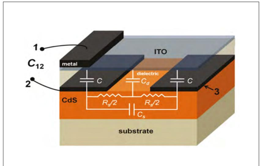
Figure 5. Internal structure of a light-dependent resistor [9]
