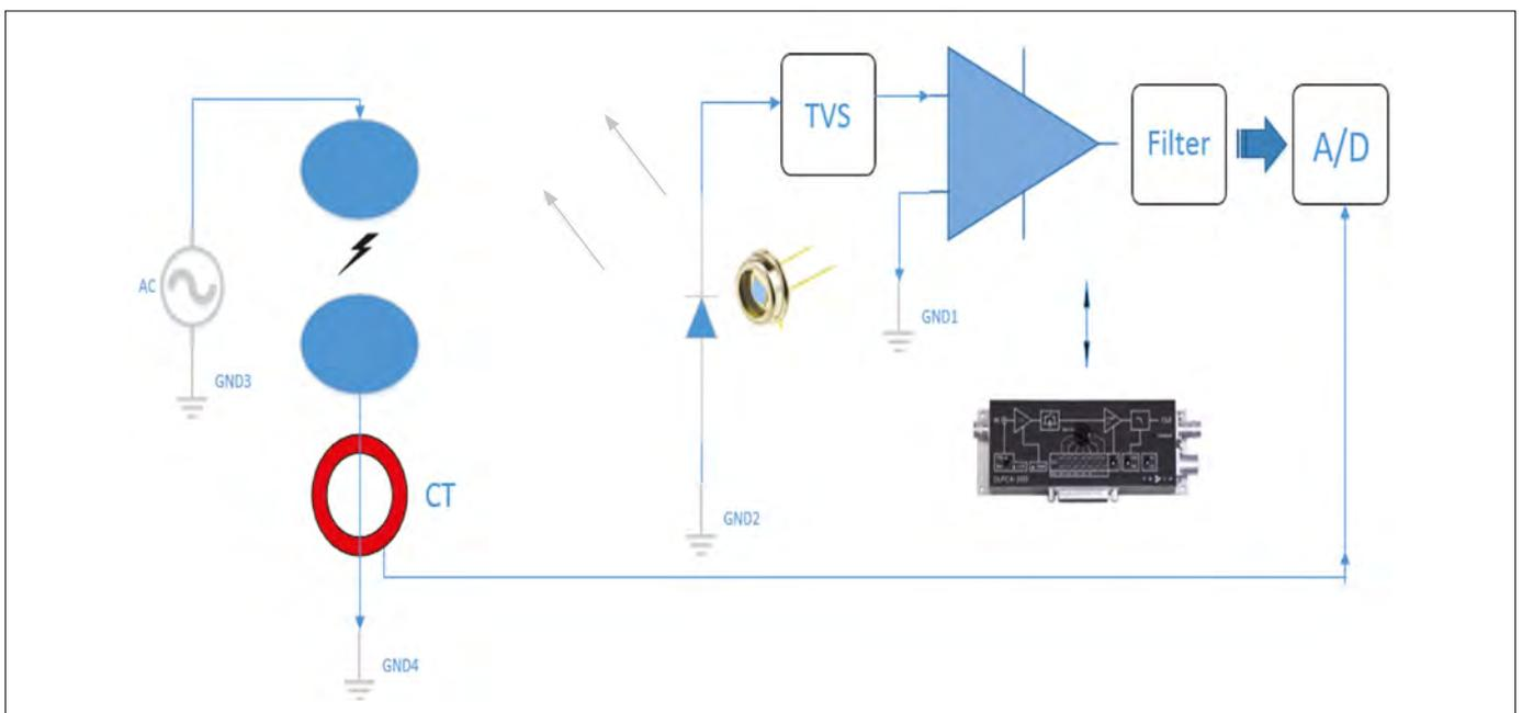
Figure 8. A schematic of the measuring circuit used for photodiodes
