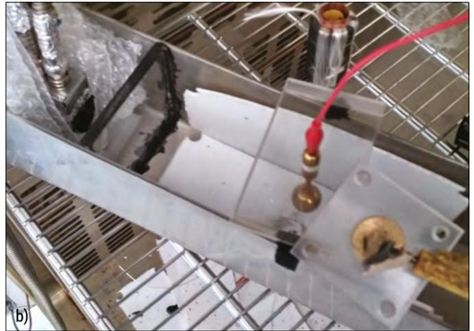
Figure 9. Some parts of the measuring circuit as for photodiodes a) Two pairs of photodiodes in a shield box, b) The measuring chamber
