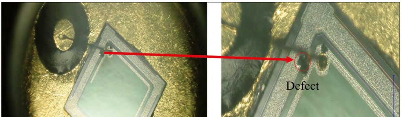
Figure 24. The substrate of a photodiode with certain defects due to proximity to the electric arc
