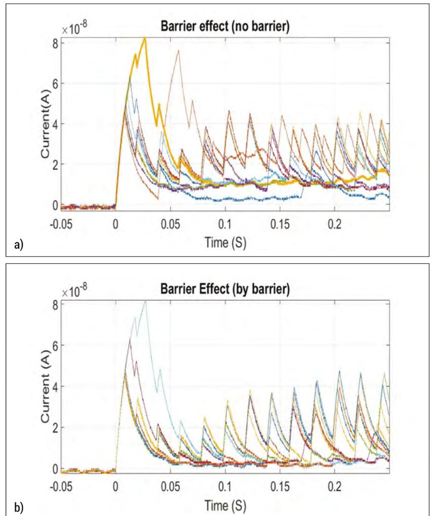
Figure 18. a) the recorder signals when the barrier was not placed. b) when the barrier was placed
