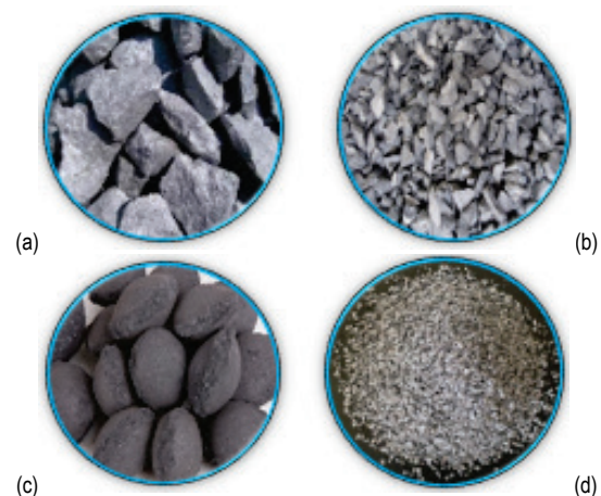
Figure 1 Silicon-based (light) master alloys as nodulizer (a) magnesium-ferrosilicon lump; (b) magnesium-ferrosilicon granular; (c) magnesium-ferrosilicon briquette; (d) magnesium-ferrosilicon powder
