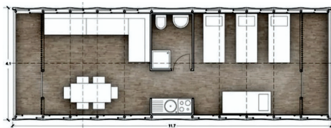
Figure 2 Temporary shelter for earthquake victims in Nepal, Barberio Colella Arc, 2013, visualization and layout
