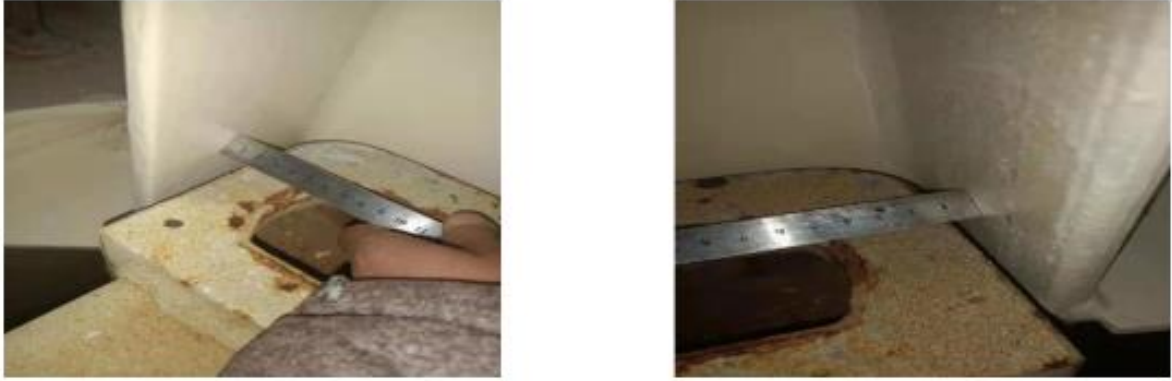
Fig. 11 Measuring the distance between the container and the cell guide
