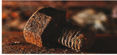
Fig. 1 Example of uniform corrosion
