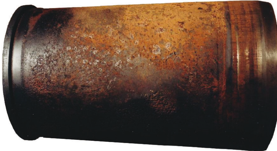
Fig. 2 Corrosion wear of combustion engine cylinder liner
