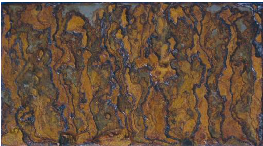
Fig. 3 Example of sample surface after corrosion test
