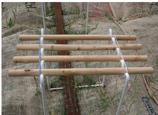
Figure 2. Samples sticks for testing the dead fuel moisture content (DFMC)
