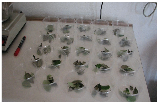
Figure 1. Samples of testing the live fuel moisture content (LFMC)
