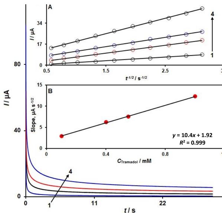
**Figure 5.** Chronoamperograms obtained at La<sup>3+</sup>/ZnO NFs-MWCNTs/SPE in 0.1 M PBS (pH 7.0) for different concentration of tramadol (1–4 correspond to 0.1, 0.4, 0.55, and 1.0 mM of tramadol). Insets: (A) plots of *I* vs. *t*<sup>-1/2</sup> obtained from chronoamperograms 1–4; (B) plot of slopes of straight lines against tramadol concentration
