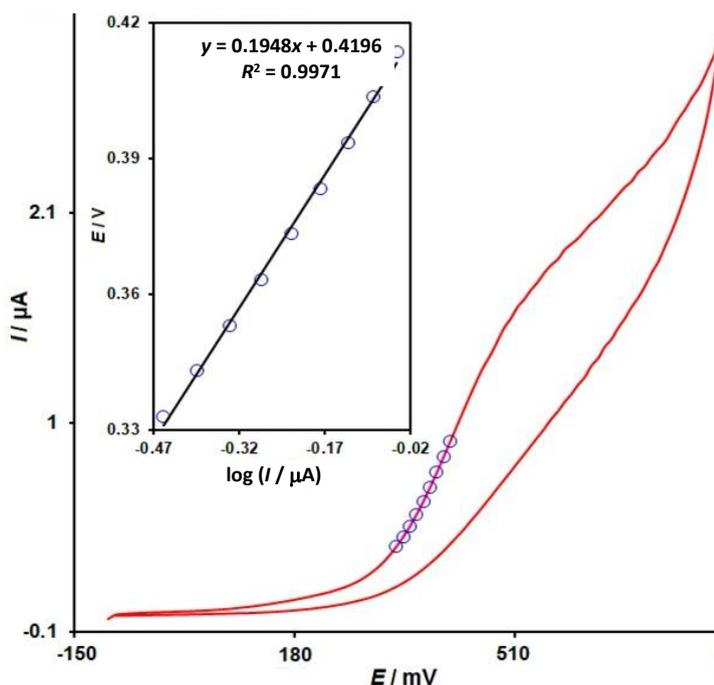
**Figure 4.** Cyclic voltammogram ( $5 \text{ mV s}^{-1}$ ) of electrode in 0.1 M PBS (pH 7.0) containing 500.0  $\mu\text{M}$  tramadol. The inset shows the Tafel plot derived from data denoted at raising part of CV
