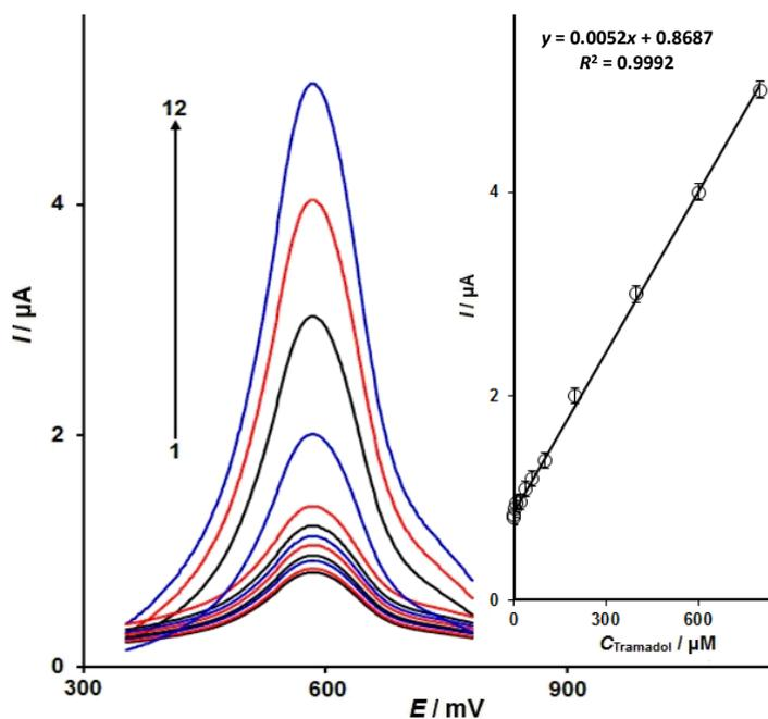
**Figure 6.** DPVs of La<sup>3+</sup>/ZnO NFs-MWCNTs/SPE in 0.1 M (pH 7.0) containing different concentrations of tramadol (1–12 correspond to 0.5, 1.0, 10.0, 20.0, 30.0, 40.0, 60.0, 100.0, 200.0, 400.0, 600.0 and 800.0 μM of tramadol). Inset: plot of the peak current vs. tramadol concentration in the range of 0.5–800.0 μM
