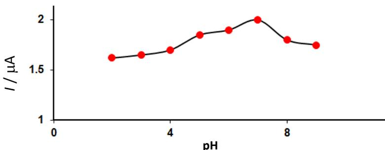
**Figure 1.** Plot of  $I_p$  vs. pH taken from DPVs of  $La^{3+}/ZnO$  NFs-MWCNTs/SPE in 0.1 M PBS containing 200.0 μM of tramadol at different pH(2.0, 3.0, 4.0, 5.0, 6.0, 7.0, 8.0 and 9.0).
