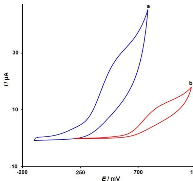
**Figure 2.** Cyclic voltammograms of (a)  $La^{3+}/ZnO$  NFs-MWCNTs/SPE and (b) bare SPE in 0.1 M PBS (pH 7.0) in presence of 400.0 μM tramadol at the scan rate 50  $mV s^{-1}$
