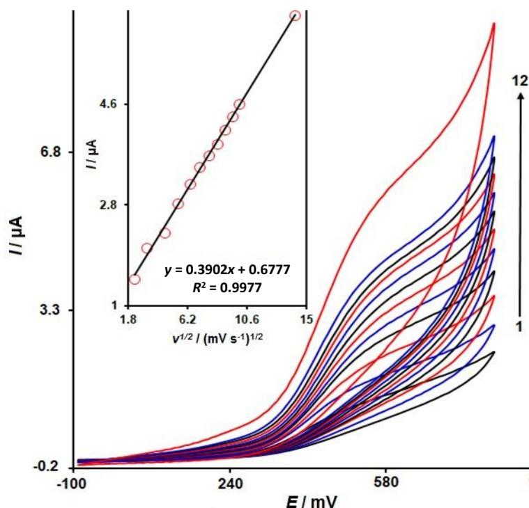
**Figure 3.** Cyclic voltammograms of  $\text{La}^{3+}/\text{ZnO}$  NFs-MWCNTs/SPE in 0.1 M PBS (pH 7.0) containing 500.0  $\mu\text{M}$  tramadol at various scan rates (numbers 1-12 correspond to 5, 10, 20, 30, 40, 50, 60, 70, 80, 90, 100 and 200  $\text{mV s}^{-1}$ ). Inset: variation of anodic peak current vs.  $v^{1/2}$
