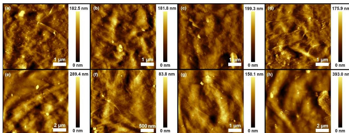
**Figure 2.** AFM (intermittent contact mode) images of graphene paper surfaces after enzyme immobilization, where EG with  $\beta$ -galactosidase enzymes are shown in: a) 0.5 mg mL<sup>-1</sup>, b) 2.5 mg mL<sup>-1</sup>, c) 5.0 mg mL<sup>-1</sup> and d) 10.0 mg mL<sup>-1</sup>, and GO with  $\beta$ -galactosidase enzymes are shown in: e) 0.5 mg mL<sup>-1</sup>, f) 2.5 mg mL<sup>-1</sup>, g) 5.0 mg mL<sup>-1</sup> and h) 10.0 mg mL<sup>-1</sup>.
