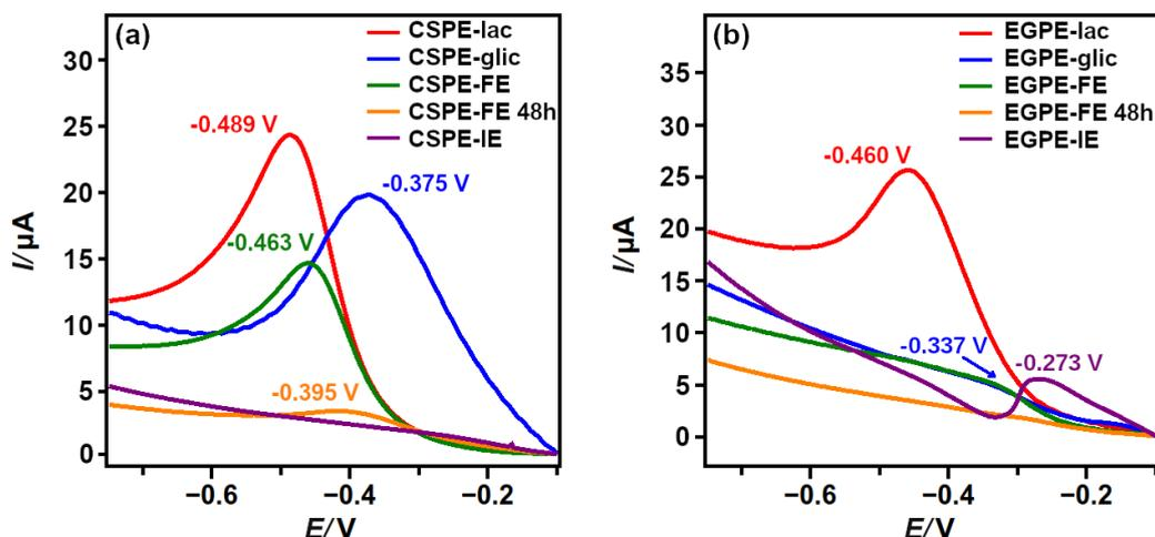
**Figure 5.** Normalized voltammograms of CSPE (a) and EGPE (b) in: pure lactose solution (red), pure glucose solution (blue), lactose solution with free enzyme (green), lactose solution with free enzyme after 48 h of reaction (orange) and lactose with immobilized enzyme (purple)
