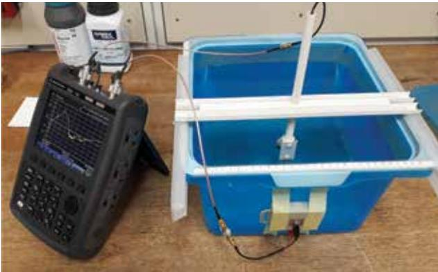
**Figure 3.** Measurement setup for implantable to on-body channel measurements on a muscle tissue equivalent liquid phantom.
