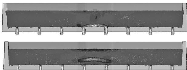
**Figure 7** The flow field in the central section of the submerged nozzle
