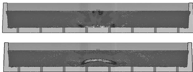
**Figure 6** The flow field in the inner section of the submerged nozzle
