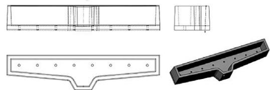
Figure 1 The tundish model
