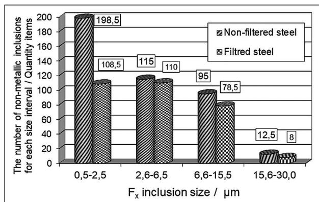
**Figure 2** The effectiveness of removing non-metallic inclusions as measured with the average rate of non-metallic inclusion number variation  $h_{\text{NMI}}$ , with division into inclusion size intervals according to  $F_x$  Feret diameters.
