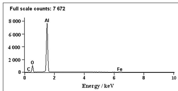
**Figure 5** X-ray photograph of non-metallic inclusions chemical composition identified on the surface of a ceramic filter and in steel volume from melt – P250GH steel.
