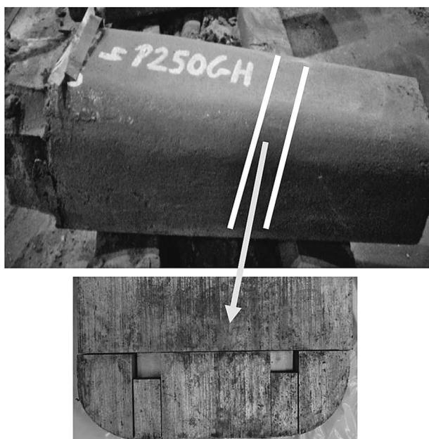
Figure 1 Places and method of sampling filtered steel.
