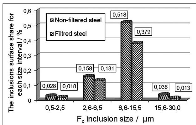
**Figure 3** The effectiveness of removing non-metallic inclusions as measured with the average rate of non-metallic inclusion superficial share  $h_{\text{NMI}}$ , with division into inclusion size intervals according to  $F_x$  Feret diameters.
