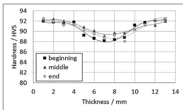
Figure 1 Collective data of Vickers hardness tests of AlCu<sub>4,5</sub>Mg<sub>3</sub> cast rods
