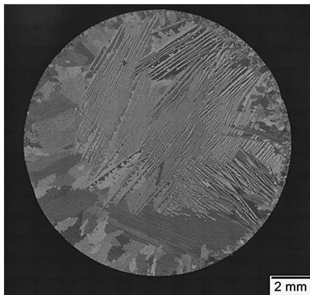
Figure 2 Macrostructure of AlCu<sub>4,5</sub>Mg<sub>3</sub> cast rod
