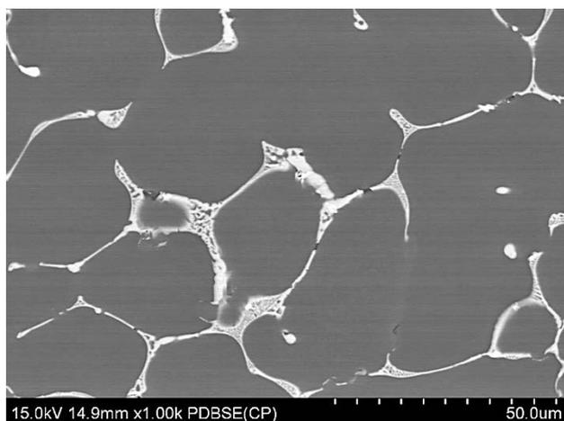
**Figure 3** Microstructure of AlCu<sub>4</sub>,5Mg<sub>3</sub> cast rod (SEM)
