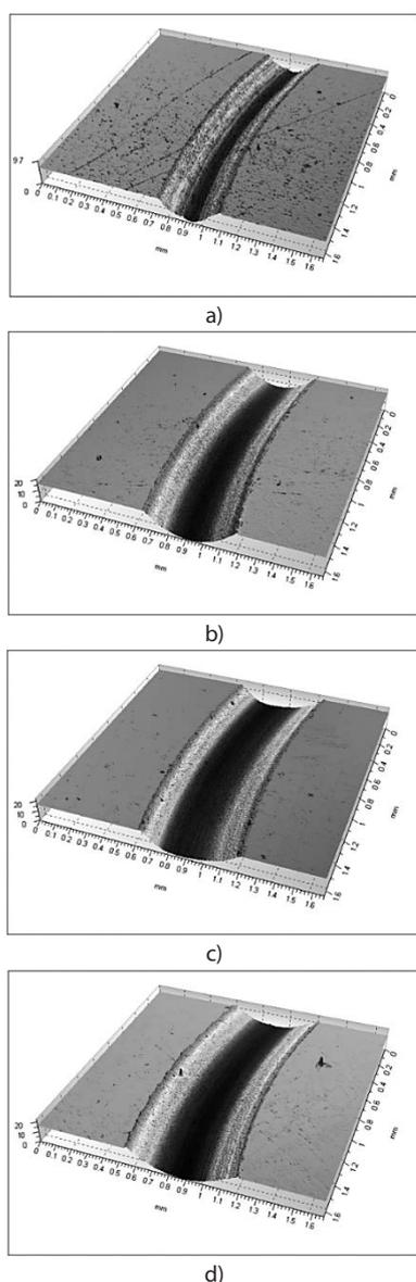
**Figure 3** Examples of abrasion wear track images obtained with profilometer, a) 1\_200, b) 1\_550, c) 1\_w\_200, d) 1\_w\_550
