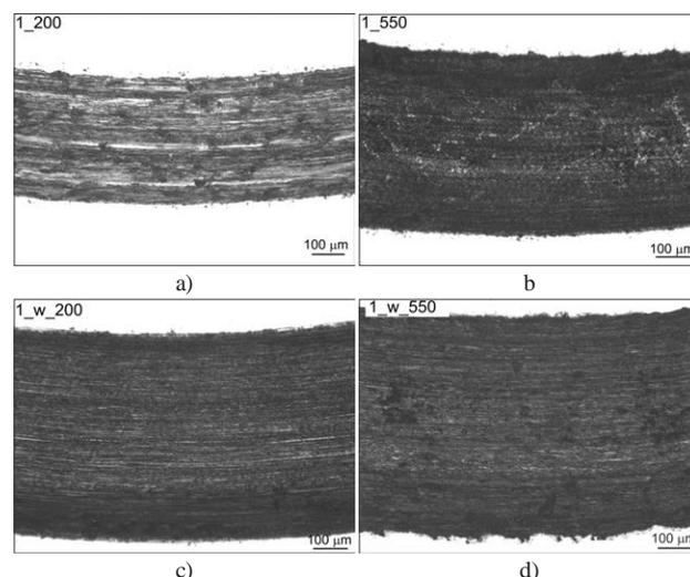
Figure 2 Examples of abrasion-wear track images obtained on surfaces of tested samples
