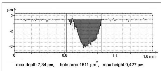
**Figure 4** Example of wear-track profile in sample 1\_200 (S1)
