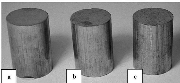
**Figure 1** Billets ( $\text{\O}40 \times 60$  mm) prepared for KOBO extrusion process; a) Pure dendritic Cu – reference sample, b) Cu + 0,2 wt. % of MWCNTs, c) Cu – 1 wt. % of MWCNTs
