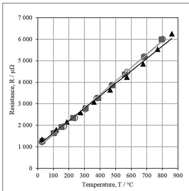
**Figure 4** Resistance characteristics in function of temperature for tested materials
