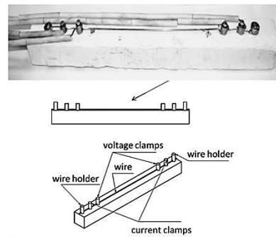
**Figure 3** Stand for electrical resistance measurements in elevated temperatures
