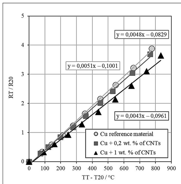
**Figure 5** Graphical interpretation of thermal coefficient of resistance for analyzed materials
