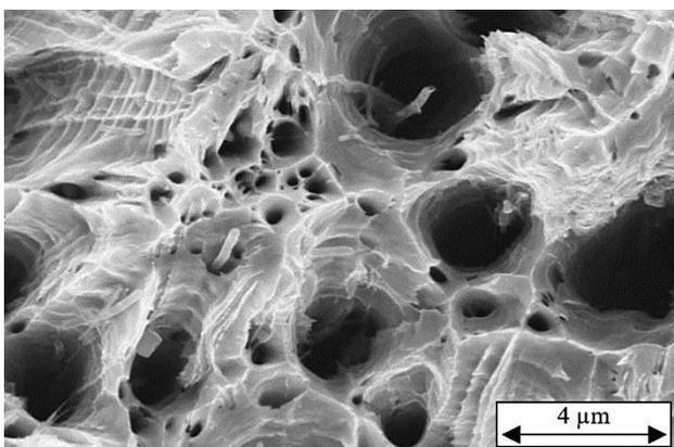
**Figure 2** SEM characterization of Cu + 1 wt. % of MWCNTs rod fracture with visible homogenous dispersion of MWCNTs and alignment of carbon nanoparticles in extrusion direction
