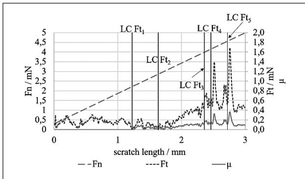
**Figure 1** Scratch test results - graph of variation of loading force (Fn), coefficient of friction (μ), friction force (Ft)
