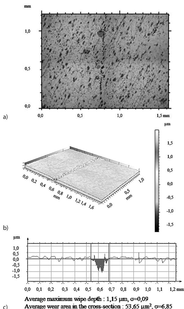
**Figure 8** Optical and axonometric views of sample wear track (a, b) and the wear profile on transverse cross-section (c) after the RS-lubricated sliding of Ti13Nb13Zr TiO<sub>2</sub>—Al<sub>2</sub>O<sub>3</sub> friction pair.
