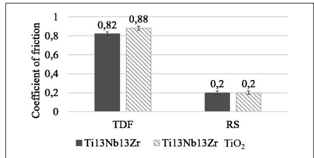
**Figure 4** Average friction coefficient obtained under dry friction (TDF) and with the use of Ringer's solution (RS) as a lubricant.
