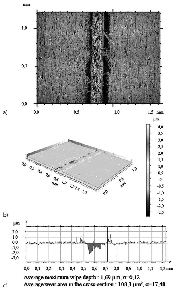
**Figure 5** Optical and axonometric views of sample wear track (a, b) and the wear profile on transverse cross-section (c) after the dry sliding of Ti13Nb13Zr—Al<sub>2</sub>O<sub>3</sub> friction pair.
