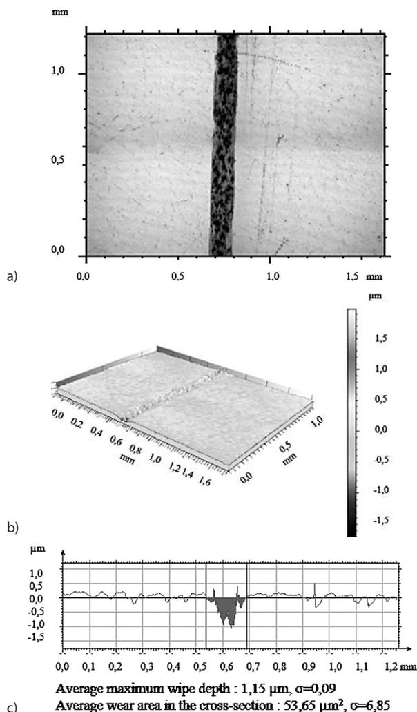
**Figure 6** Optical and axonometric views of sample wear track (a, b) and the wear profile on transverse cross-section (c) after the RS-lubricated of Ti13Nb13Zr — Al<sub>2</sub>O<sub>3</sub> friction pair.
