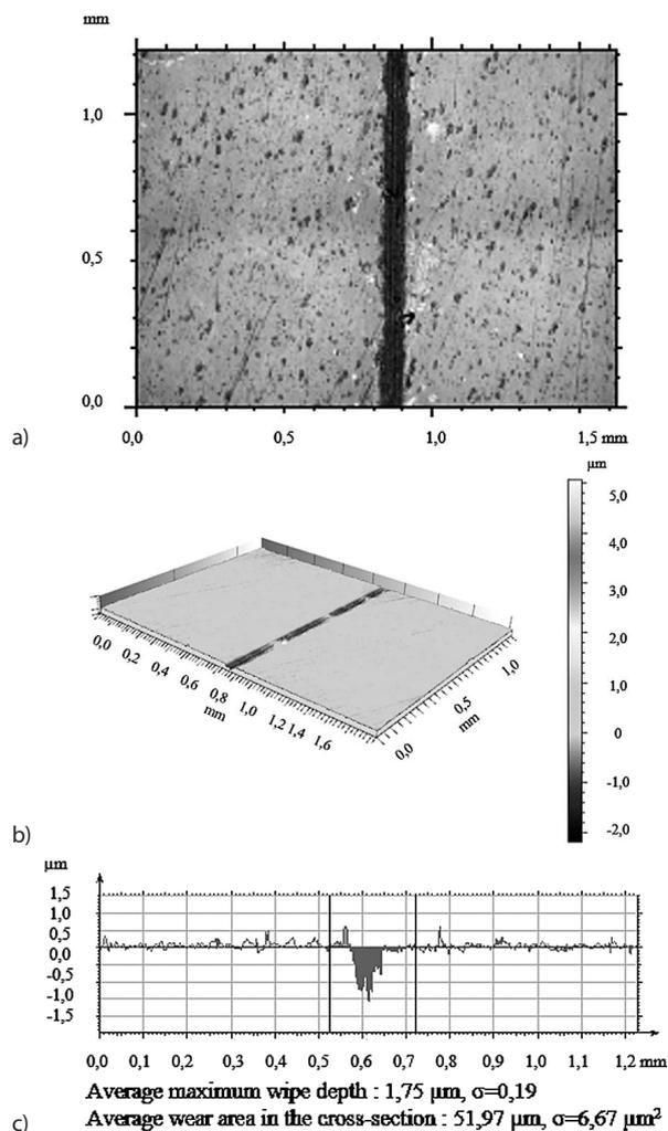
**Figure 7** Optical and axonometric views of sample wear track (a, b) and the wear profile on transverse cross-section (c) after the dry sliding of Ti13Nb13Zr TiO<sub>2</sub> — Al<sub>2</sub>O<sub>3</sub> friction pair.
