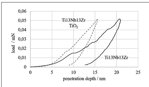
**Figure 3** Load – penetration depth curves from indentation tests
