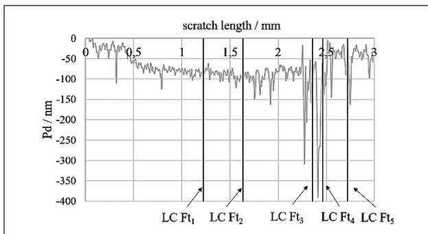
**Figure 2** Scratch test results - penetration depth of the indenter (Pd)
